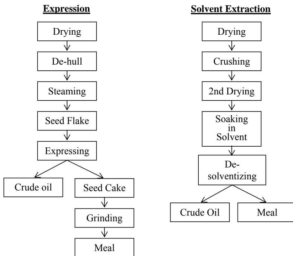
**Figure 1.3** Flow Sheet for Crude Tea Seed Oil Extraction by Expression and Solvent
