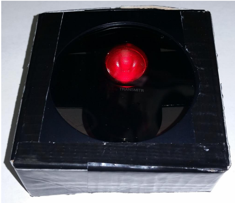
Figure 1.2: A Bontrager Flare RT inside a custom-made neutral density (ND) filter box mount, which holds the 0.3 ND filters in front of the light in order to reduce the luminance of the taillight in half. The circular frame on the box is the mechanism that holds the ND filter in place.
