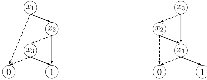
Figure 3.2: Two BDDs of f = x_1x_2x_3 + x_1x_2 + x_1x_3 . The one on the left arises from the variable order x_1 < x_2 < x_3 , and the one on the right arise from x_3 < x_2 < x_1
