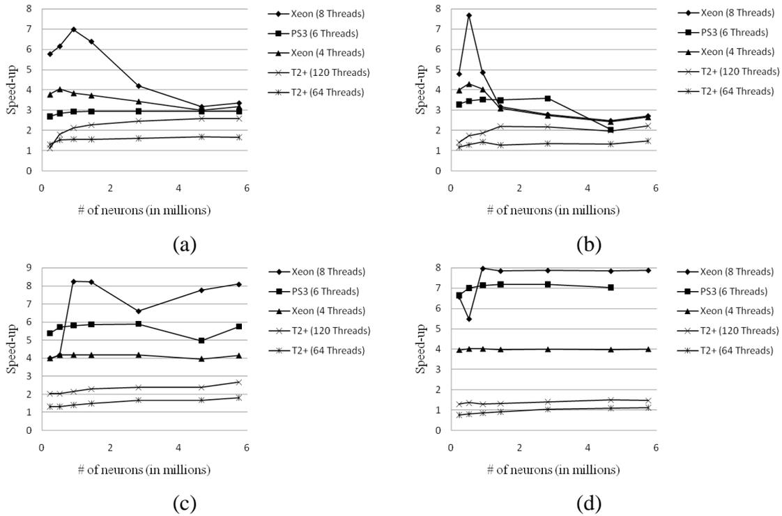
**Figure 8.1.** Speed-up for Intel Xeon E5345 platform (8 threads), Sony PS3 (6 threads), Intel Xeon E5345 platform (4 threads), Sun UltraSPARC T2+ T5140 (120 and 64 threads over vectorized Intel Xeon single thread for the (a) Izhikevich, (b) Wilson, (c) Morris-Lecar, and (d) Hodgkin-Huxley models.
