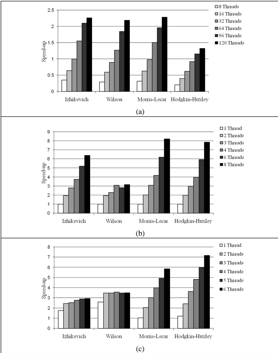
**Figure 8.3.** Variation in speed-up of the  $1200 \times 1200$  network with the number of threads for the (a) Sun UltraSPARC T2+, (b) Intel Xeon, and (c) Cell platforms.
