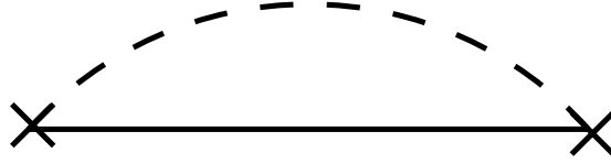
Figure 1. Second-order self-energy contribution due to magnetic impurities. The solid line represents the Green's function while the crosses describe the interaction with a single magnetic impurity.
