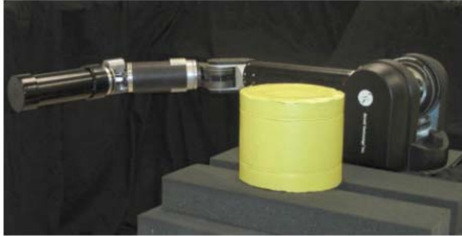
Figure 2.1: Experiment setup showing the Barrett Whole Arm Manipulator and object to be grasped
