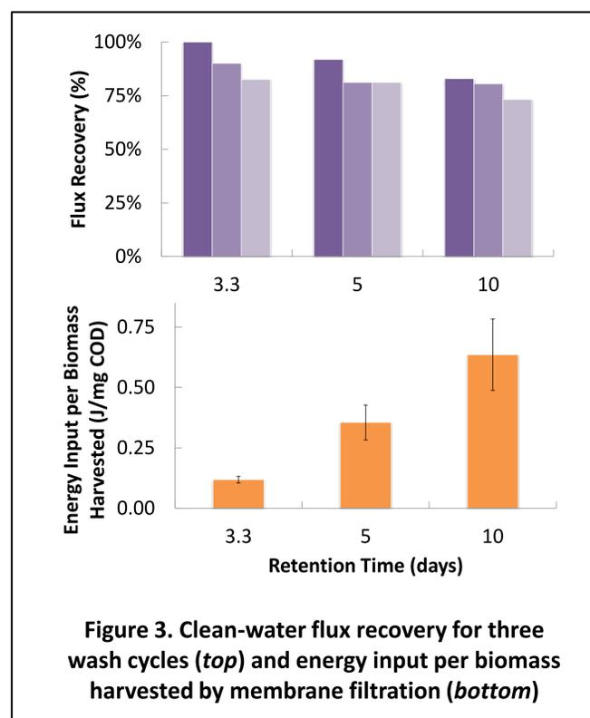
Figure 3. Clean-water flux recovery for three wash cycles (top) and energy input per biomass harvested by membrane filtration (bottom)
