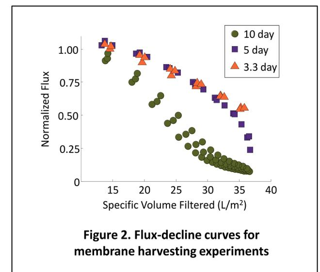
Figure 2. Flux-decline curves for membrane harvesting experiments
