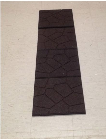
Figure 2: Mock sidewalks with the fourth paver raised 1.19 cm and gap size set to 0.64 cm.
