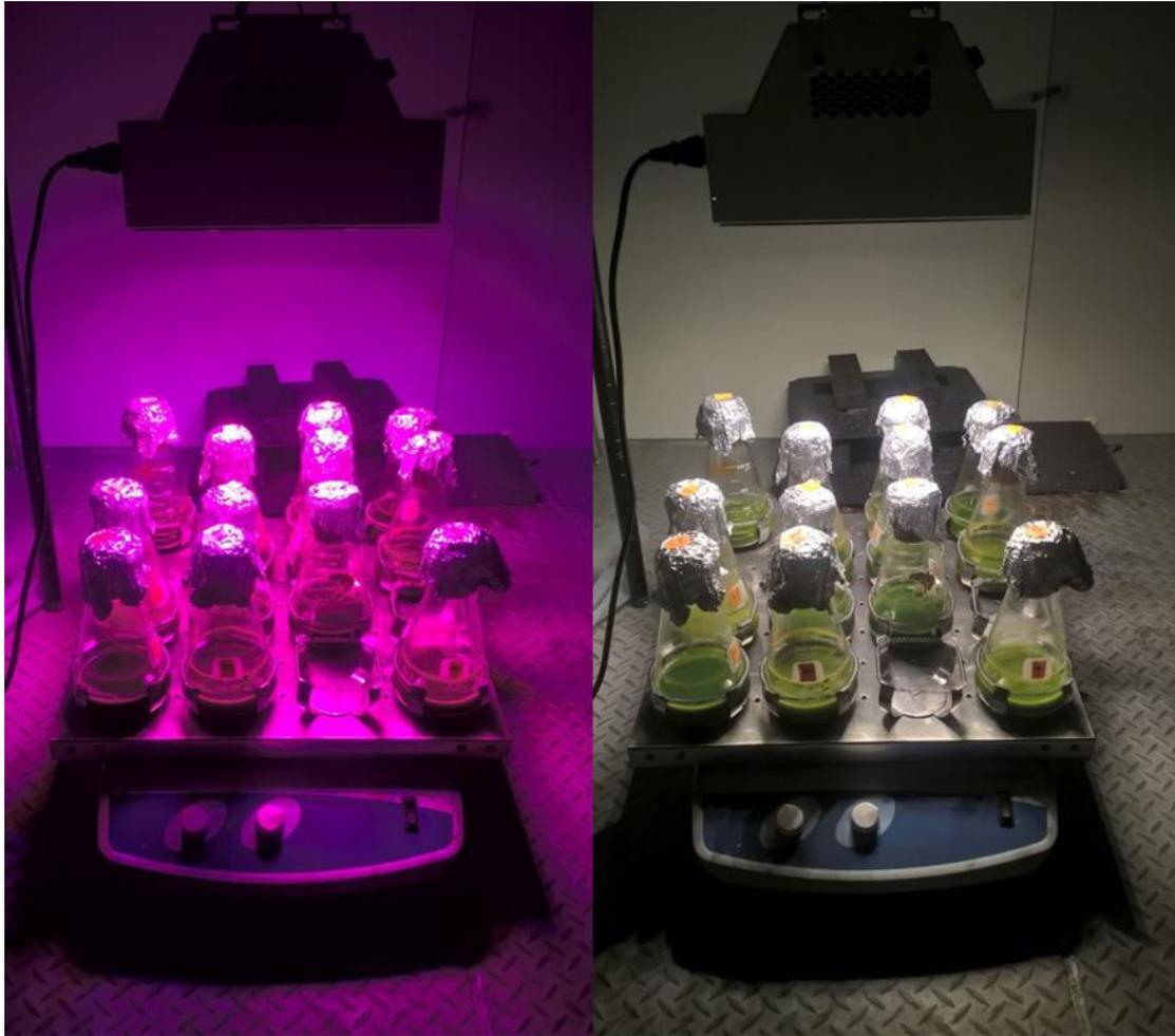
Figure B.1 Reactor setup of mixotrophic *Chlorella protothecoides* cultures in the dark room. Left, LED light was turned on; Right, the light source was toggled to white light.
