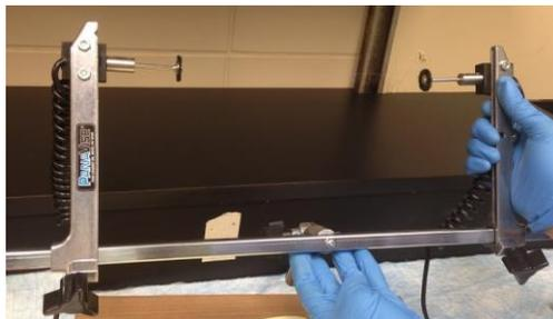
*Scheme 5. Custom-made fiber collector and twisting device*
