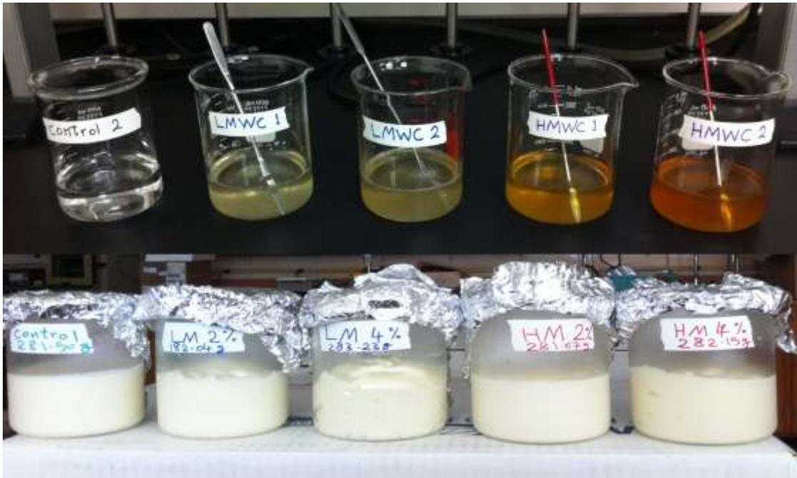
**Figure 3.2:** Low and high molecular weights water soluble chitosan with WMP treatments.
