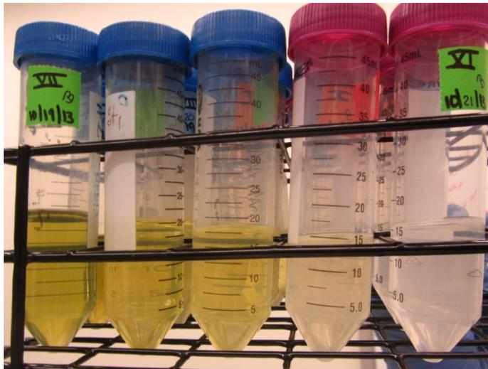
Figure 3.4.1 Extracted lipids in hexane solvent for Run 2. From left to right: 0, 1.5, 3, 6, and 9 hour interval heterotrophic growth lipid extractions
