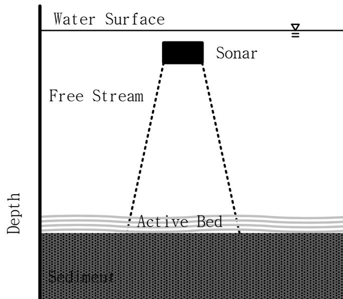
Figure 3.1: Schematic setup for the turbidity stratification test.
