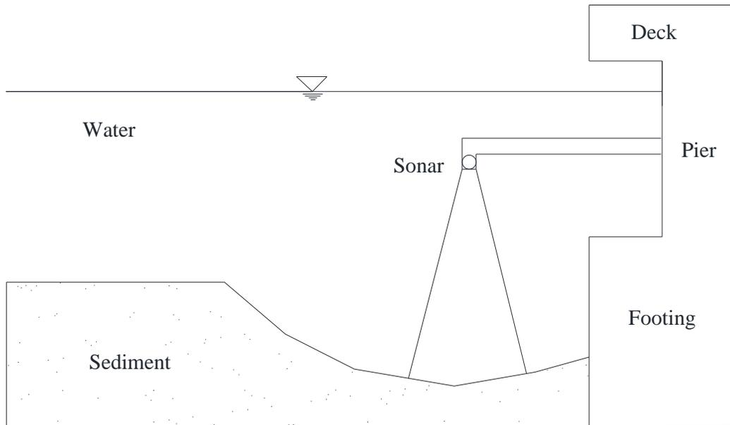
Figure 2.1: Typical installation of Sonar (Based on Nassif et al., 2002 ; Fisher 2012)
