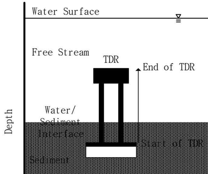
Figure 3.3: Schematic of the TDR setup.
