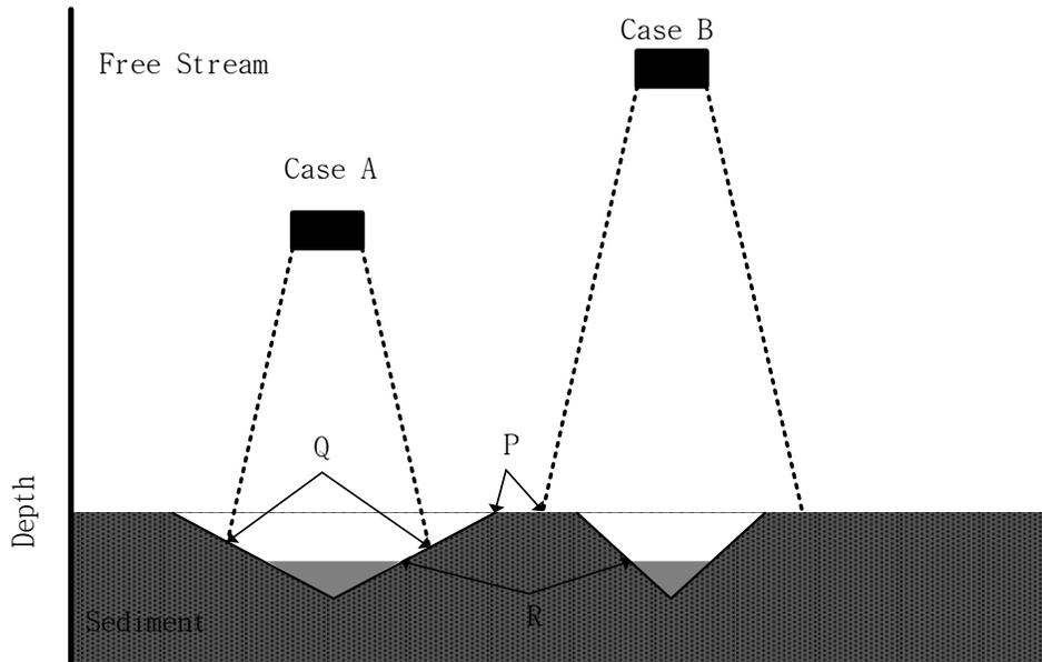
Figure 4.7: Sonar beam to scour hole size experimental setup.
