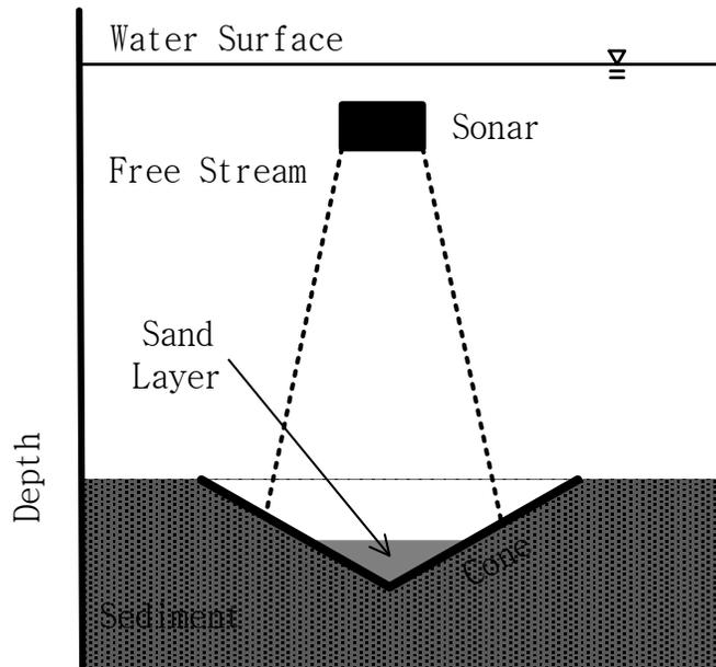
Figure 3.2: Schematic setup for the scour hole/beam ratio tests.
