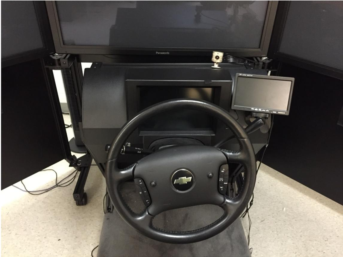
**Figure 10. Arrangement of in-vehicle display on driving simulator**
