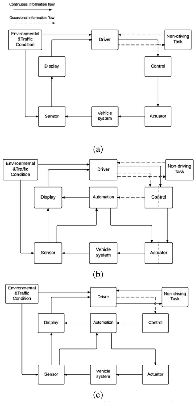
Figure 2. (a): Information flow at level 0 (within control loop); (b): Information flow at level 1 (partially out of the loop); (c): Information flow at level 2 and 3 (approximately fully out of the loop)
