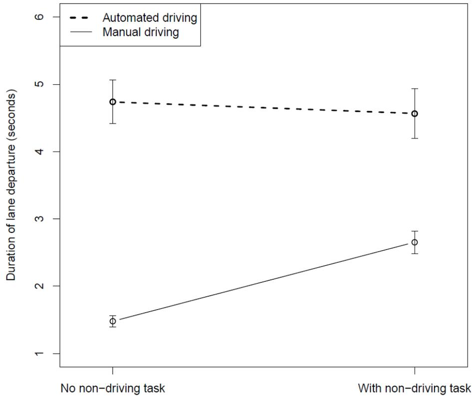
**Figure 12. Lane departure time (with standard error bars) (with standard error bars) for the with and without a non-driving task for the manually driving or the automated driving**
