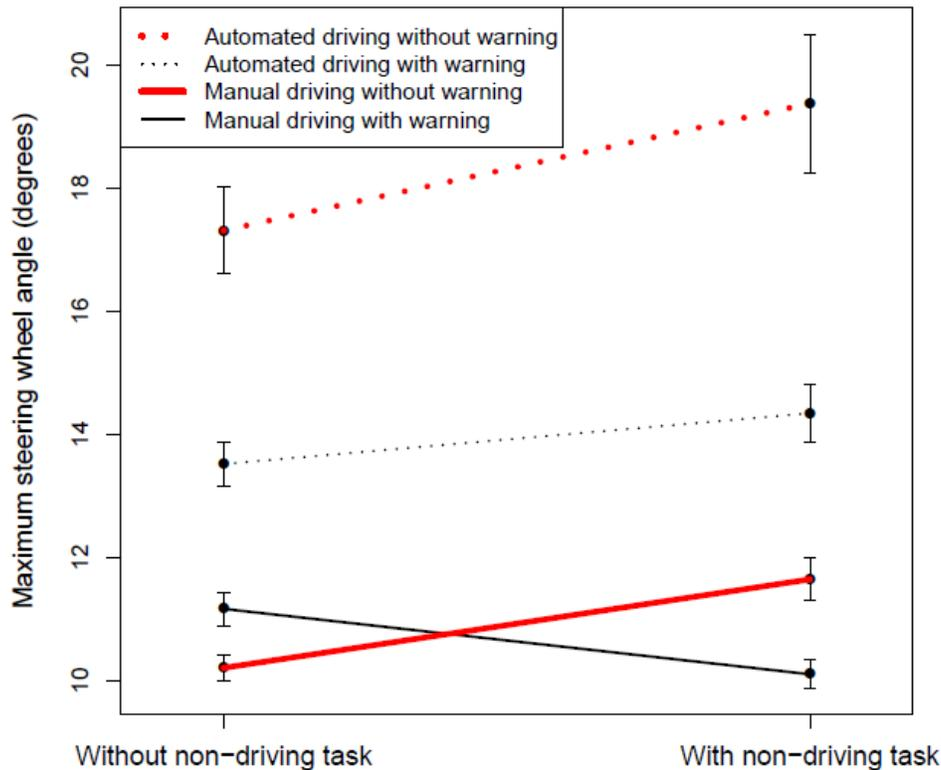
**Figure 16. Maximum steering wheel angle (with standard error bars) across automation conditions, non-driving task status, and warning conditions**
