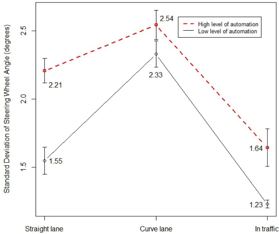
**Figure 9. Standard deviation of steering wheel angle (and standard error bars)**
