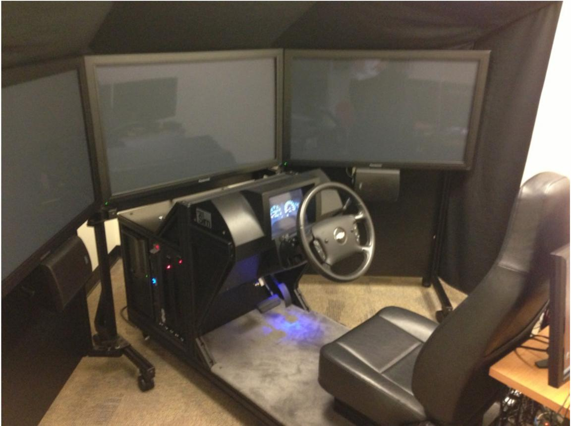
Figure 3. MinSim driving simulator
