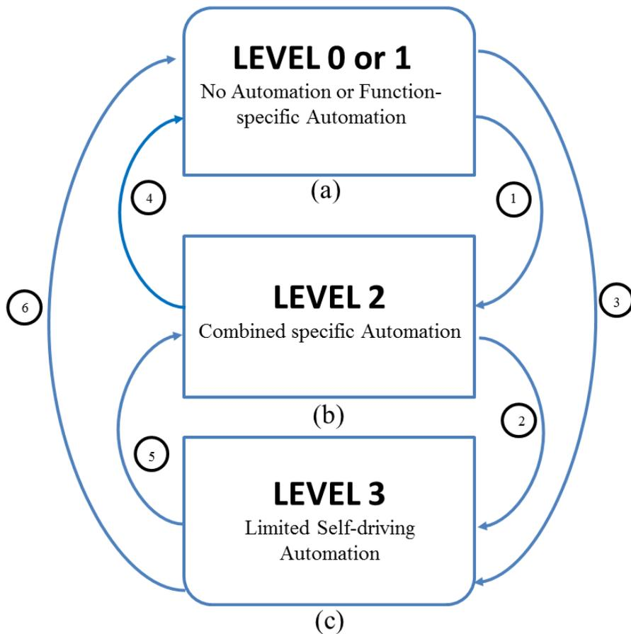
**Figure 17. The transitions between each levels of automation (a) Level 0 or 1 automation; (b) Level 2 automation; (c) Level 3 automation**
