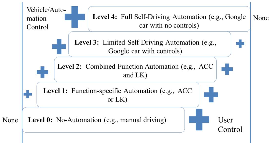
Figure 1. The NHTSA Automation levels modified from Blanco et al. (2015)
