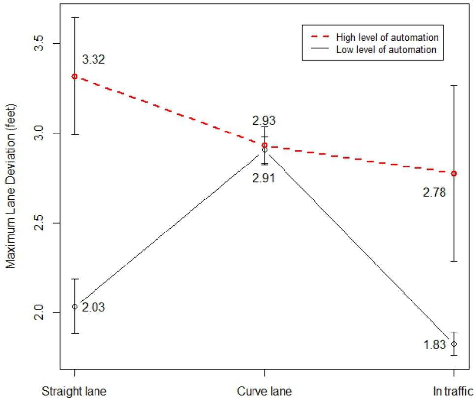
**Figure 7. Maximum lane deviation (and standard error bars)**
