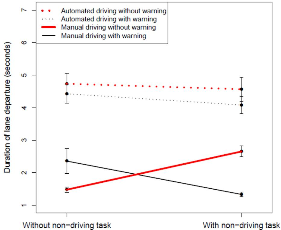
**Figure 15. Duration of lane departure (with standard error bars) across automation conditions, non-driving task status, and warning conditions**
