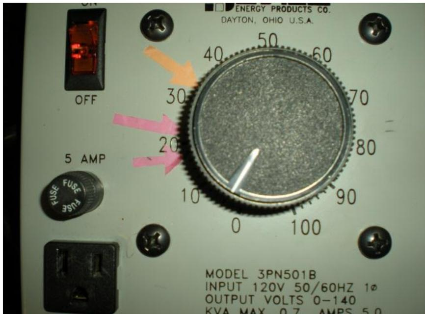
Figure 3. Variac used to manipulate glare intensity
