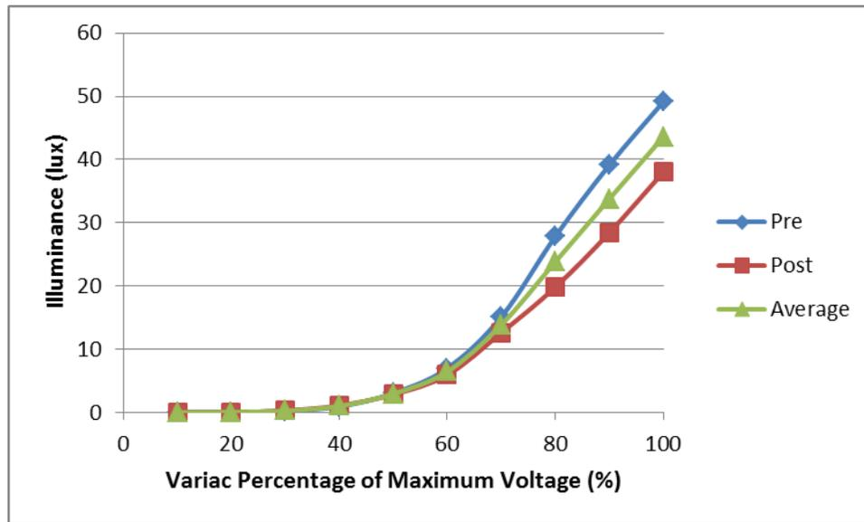
Figure 5. Pre and post experiment illuminance (lux) of the Glare Box measured at the participant's eye
