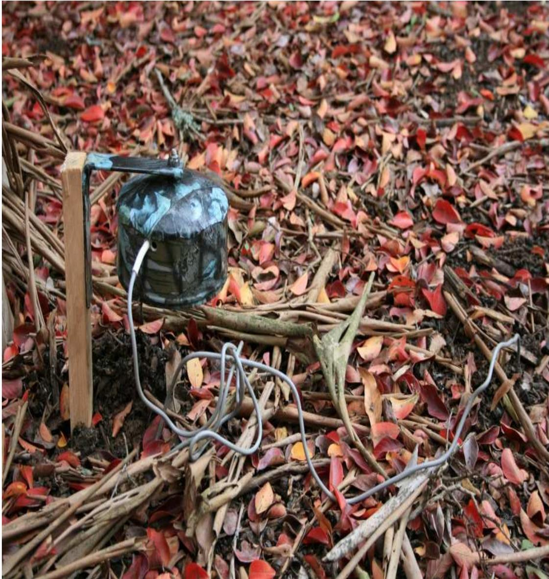
Fig. 3.1. A HOBO data logger was placed into the waterproof station at Lake Greenwood State Park. Thermocouples were attached to data loggers and placed 25 cm into an underground.
