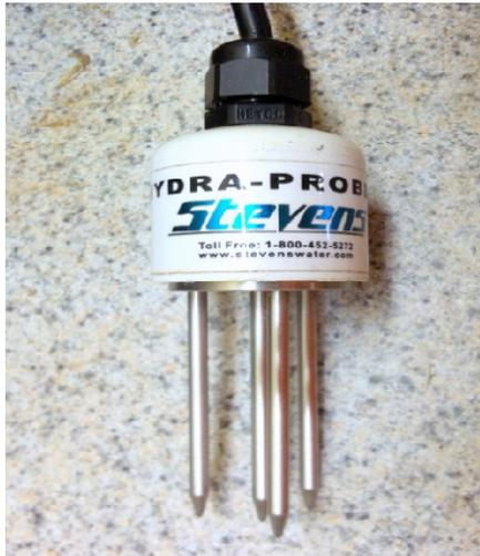
Figure 1. Commercial probe used to determine volumetric water content, soil temperature, electrical conductivity, and dielectric constant/permittivity.
