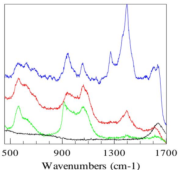
Figure 4.6. Raman spectra of silver reduced onto alumina membranes with a pore diameter of 100nm (black) via the chemical reduction of silver (I) oxide by ethanol and bubbling N<sub>2</sub> gas. The alumina membranes were plasma cleaned for 1min (blue), 5min (red), and 10min (green) prior to deposition.
