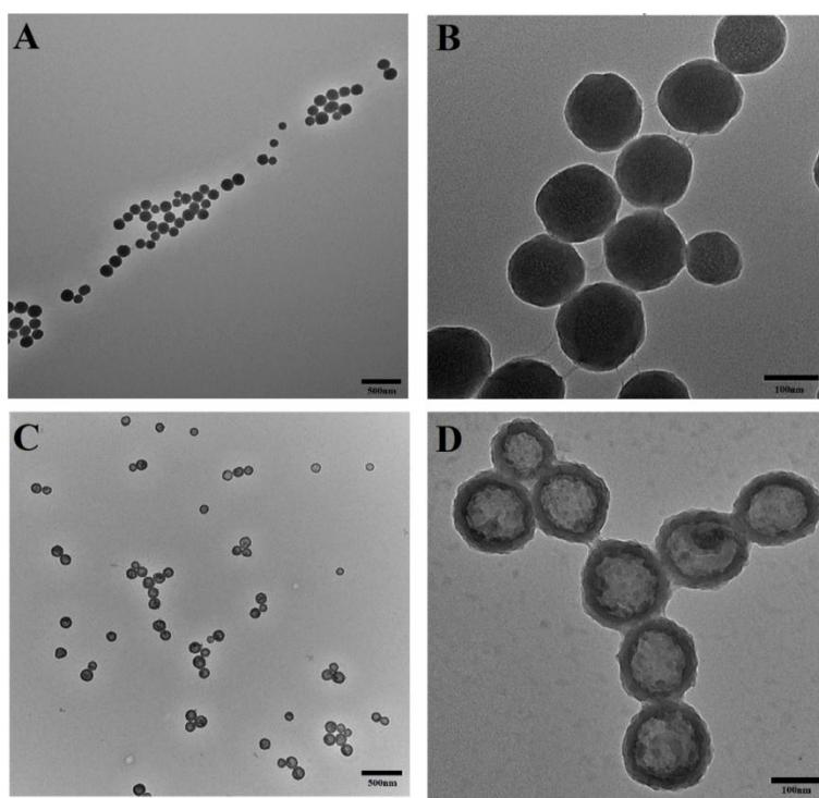
Figure 2.1. TEM images of silica/poly(4-vinyl pyridine) nanocomposites before heating (A,B) and after heating at 70°C for 4hrs (C,D).
