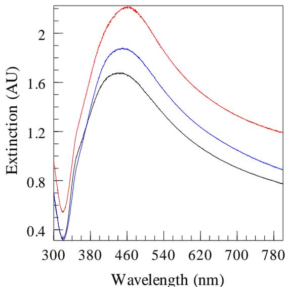
Figure 4.1. UV-Vis spectral series of silver reduced onto glass slides via the chemical reduction of silver (I) oxide by ethanol where the reaction was taken place in the dark (black), stationary in ambient light (blue) and rolling in ambient light (red).
