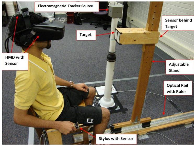
*Figure 3:* Shows our near-field distance estimation apparatus. The target, participant's head, and stylus are tracked in order to record actual and perceived distances of physical reach in the IVE
