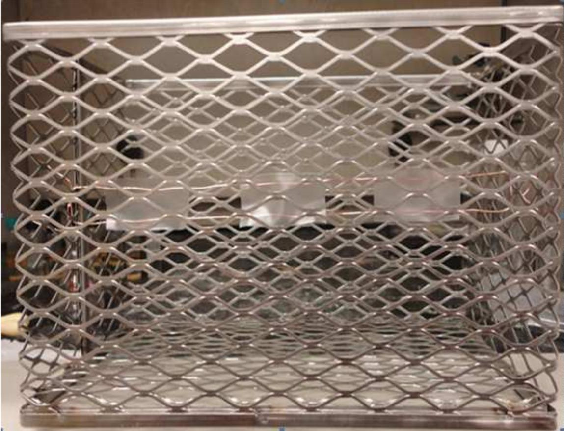
Figure 2.2. Stainless stain deploying basket. Three PEs were woven on copper wires and then attached to mesh openings of the basket
