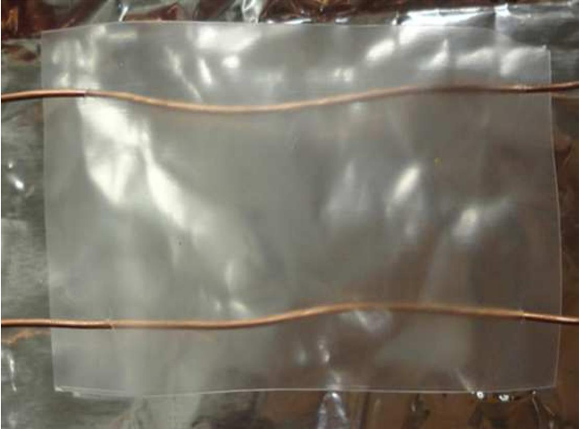
Figure 2.1. Single-layer polyethylene (PE) (5 cm long, 2.5 cm wide) used to collect dissolved PCBs.
