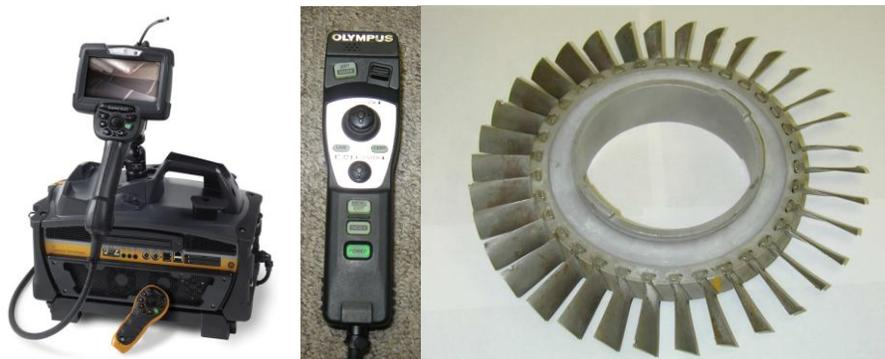
**Figure 1: Video borescope, control, and rotor (from left to right)**
