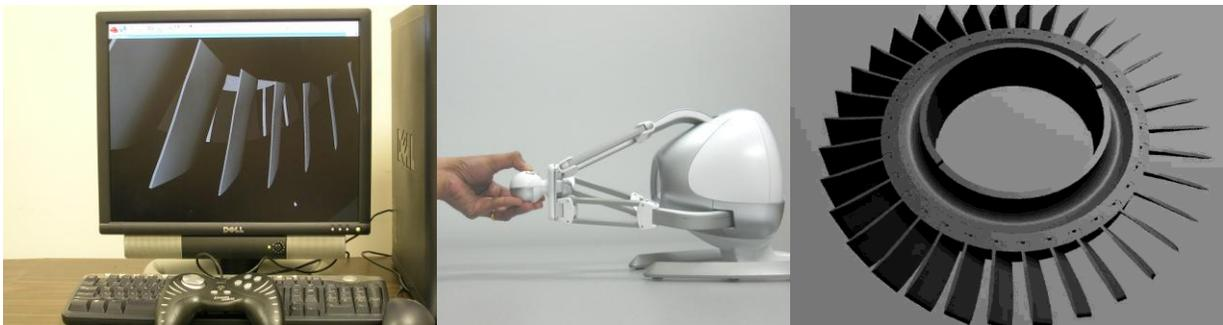
**Figure 2: Desktop with gamepad, Falcon, and rendering of rotor**
