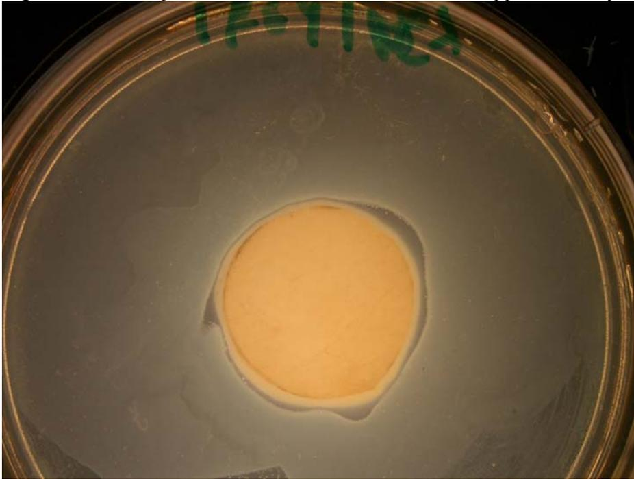
Thus, no diffusion into the surrounding media could be distinguished for any of the chitosan coated films or paper infused with chitosan. Comparing the results of film on lawn tests as well as wet/dry paper disc tests indicated that chitosan has antimicrobial activity which is effectively expressed only in aqueous systems regardless of the molecular weight of chitosan. Wet paper discs showed diffusion of chitosan into the surrounding agar.
