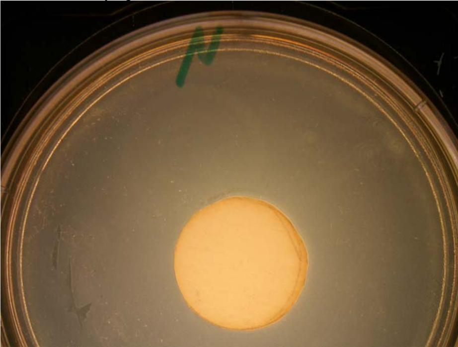
Figure 14. Wet Paper Disk with a Diameter of 25 mm dipped in 1 kGy Chitosan Solution
