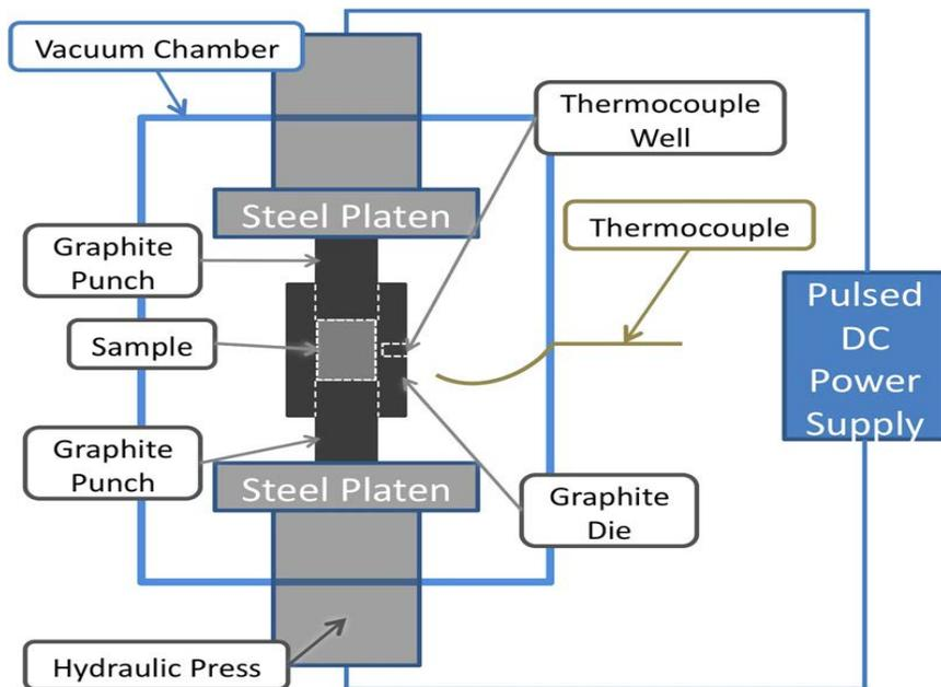
Fig. 1 Dr. Sinter specimen chamber. The thermocouple (TC) is located in the vacuum chamber and for die temperature measurements the TC is placed in a hole in the die. The TC is located in the vacuum chamber external to the die for measurements with the spectrum analyzer as an antenna (TCa).
