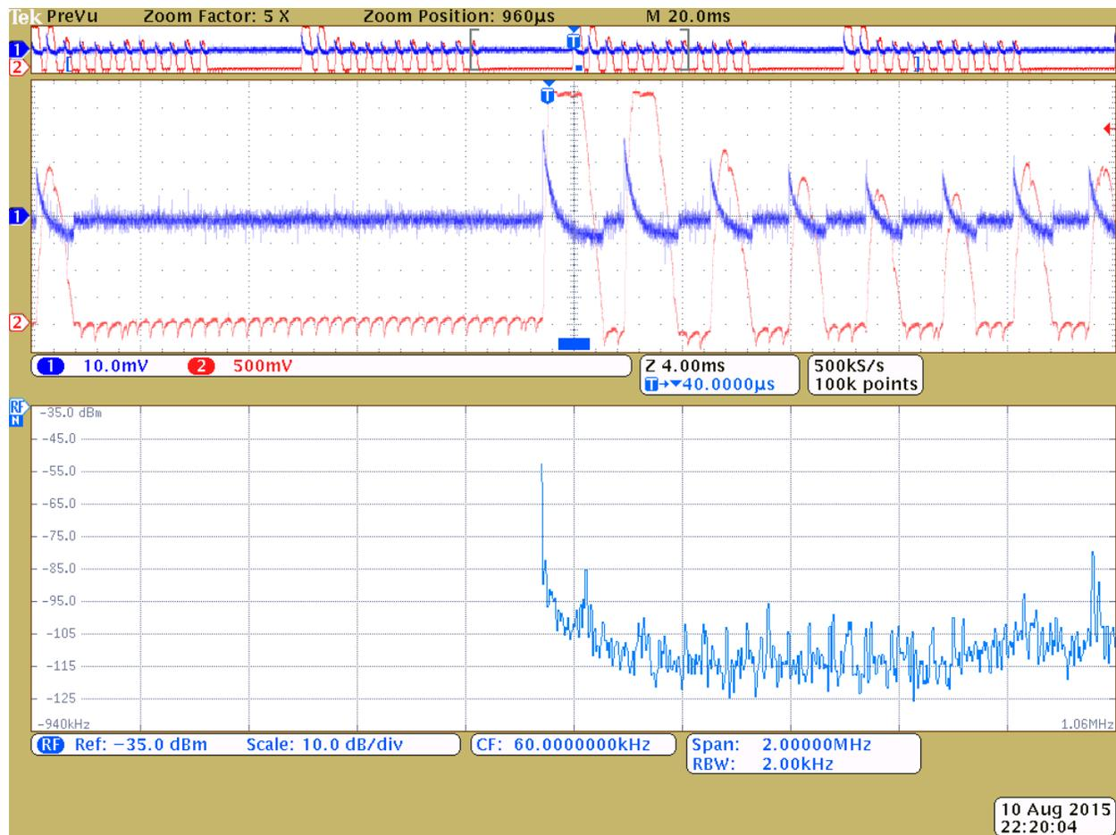
Fig. 2 B Colors and traces as shown in Fig. 2 A. The blue bar of the middle panel is shifted to include the pulse peak and initial shut off of the PECS current. From the peak at about 12 kHz in Fig. 2 a drop of 45 dBm is observed.
