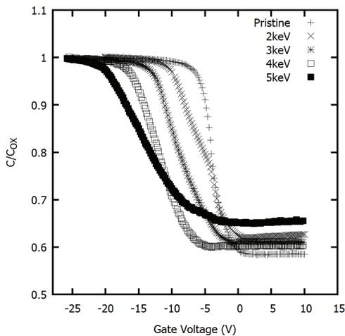
Fig. 3. Irradiated device CV curves (HF) for devices exposed to  $\text{Na}^+$  ions in the range of 2 keV to 5 keV. The capacitance values have been normalized by  $C_{\text{ox}}$ .
