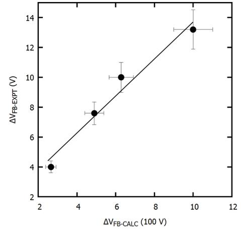
Fig. 6. Calculated  $\Delta V_{FB-CALC}$  assuming no recombination plotted with the measured flatband shifts,  $\Delta V_{FB-EXPT}$ . The slope obtained by a linear fit ( $1.2 \pm 0.2$ ) is a measure of the holes lost to recombination.
