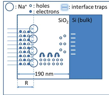
Fig. 4. A schematic depicting hole creation and transport in the oxide leading to a shift in the flatband voltage and skew in the C-V curve. See text for details.
