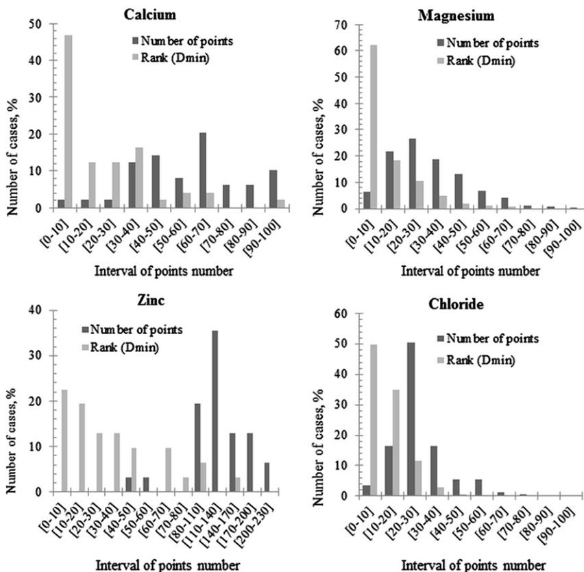
FIGURE 3 Distribution of all representative grid points found by the clustering method with Rank = 1 (*dark bars*) and the Rank of the closest representative grid point with respect to the original ion's position (*light bars*).
