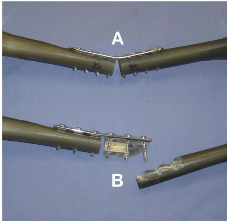
**Figure 2.2:** Mode of failure under 4-point AP bending for each implant type. A) LC plates failed via plastic deformation. B) LCDC plates failed via bony fracture through screw holes.
