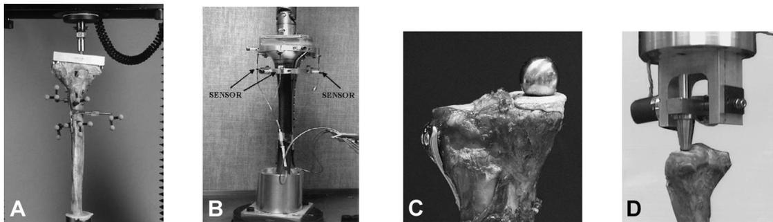
**Figure 1.4:** Load application setup from various proximal tibia fixation device evaluations depicting both physiologic and “case-specific” load conditions. A-B) Point of load application approximates physiologic load application during weight-bearing. C-D) Point of load application is “case-specific” relative to tested implant and fracture pattern. Reproduced from (left to right) Mueller et al. 2005, Peindl et al. 2004, Ratcliff et al. 2007, and Karunaker et al. 2002
