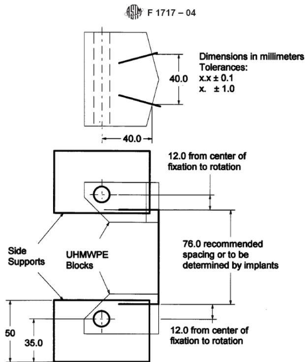
**Figure 1.1:** Lumbar Bilateral Construct Test Setup for Screws. Reproduced from ASTM F1717-04
