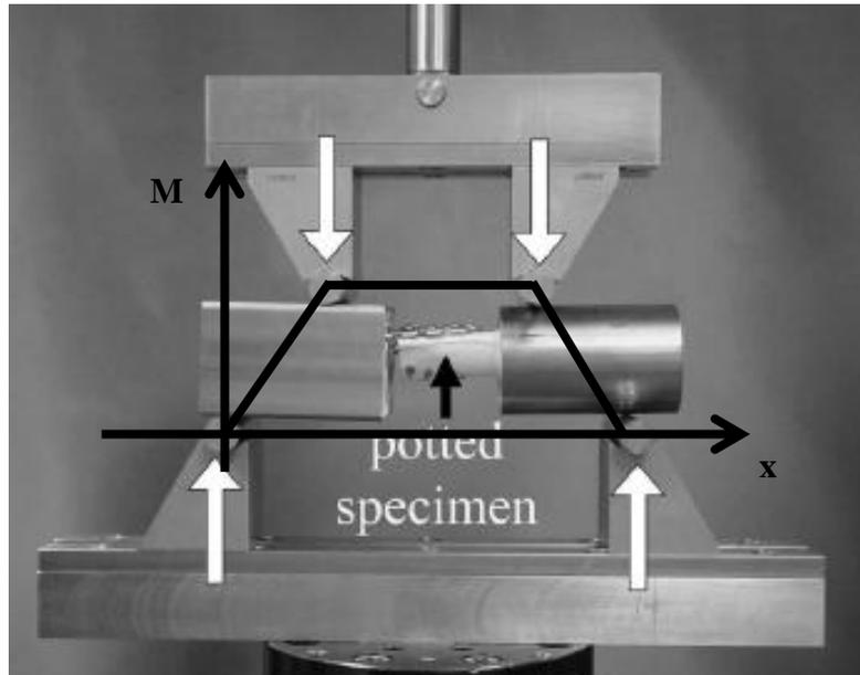
**Figure 1.6:** Four-point bending setup creates a constant moment across the region of interest. Modified from Korner et al. 2004
