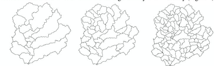
Figure 3: Subwatershed configurations (high, medium, and low density)
