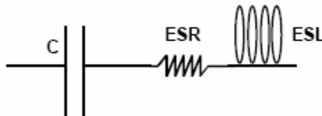
Fig 3.8 RLC Circuit representation of a capacitor [4].
