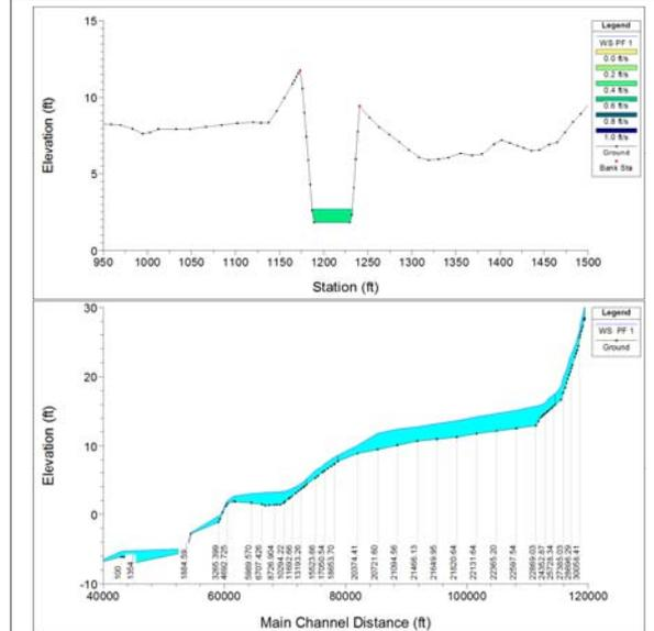
Figure 6. Steady flow simulation (cross section and profile view)
