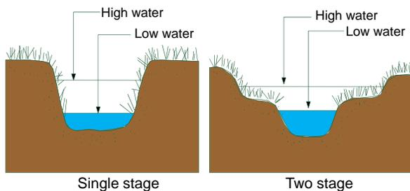
Figure 1. Single stage design vs. two stage design
