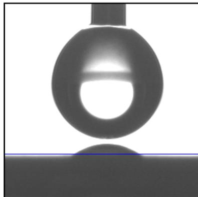
**Figure A.3.** Image of the sample being raised to the water drop.
