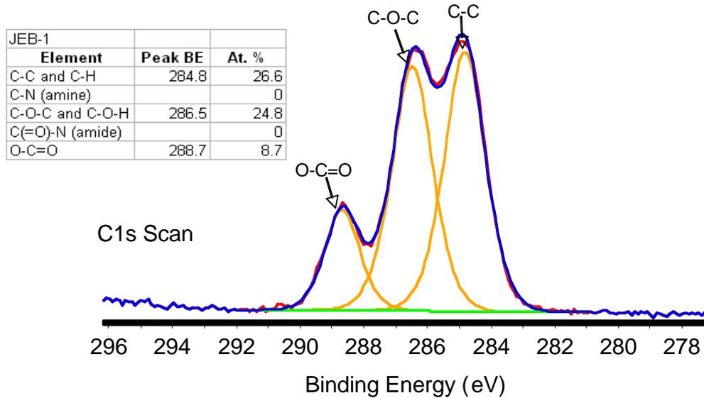
**Figure C.2.** C 1s scan of sample JEB-1 (PGMA on Si wafer).
