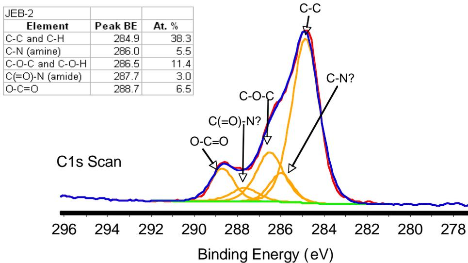
**Figure C.4.** C 1s scan of sample JEB-2 (PGMA with diamine attachment).
