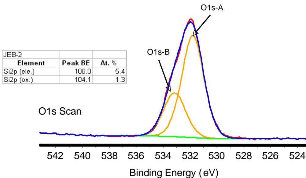
**Figure C.5.** O 1s scan of sample JEB-2 (PGMA with diamine attachment).
