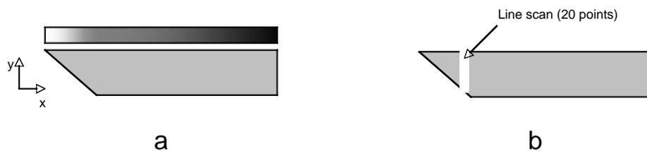
**Figure 3.7.** (a) Sample used for DOD printing the biomolecule. (b) Indicated line is placement where XPS line scan measurements shown in Figure 3.8 were made.
