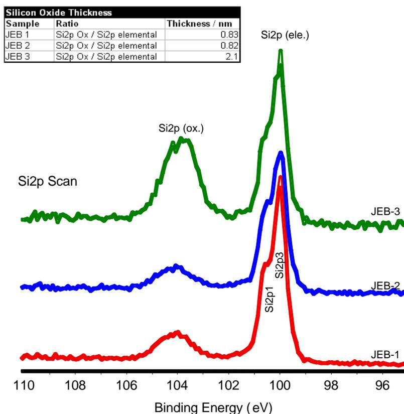
**Figure C.1.** Si signal from XPS on attachment procedure samples.
