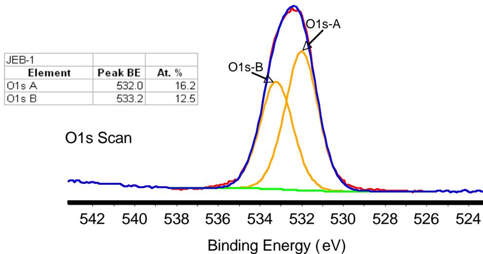
**Figure C.3.** O 1s scan of sample JEB-1 (PGMA on Si wafer).
