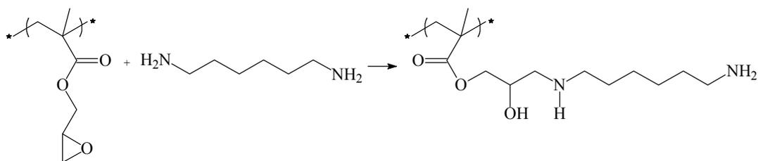
**Scheme 3.1.** Proposed result from reaction of PGMA layer with 1,6-diaminohexane, yielding a diamine-modified PGMA.
