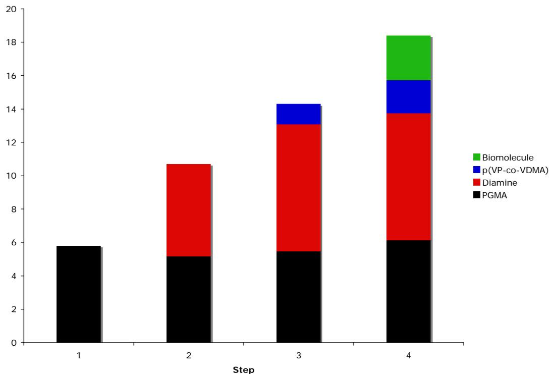
**Figure 3.1.** Ellipsometric thicknesses of each step in the preparation of multilayer scaffold.
