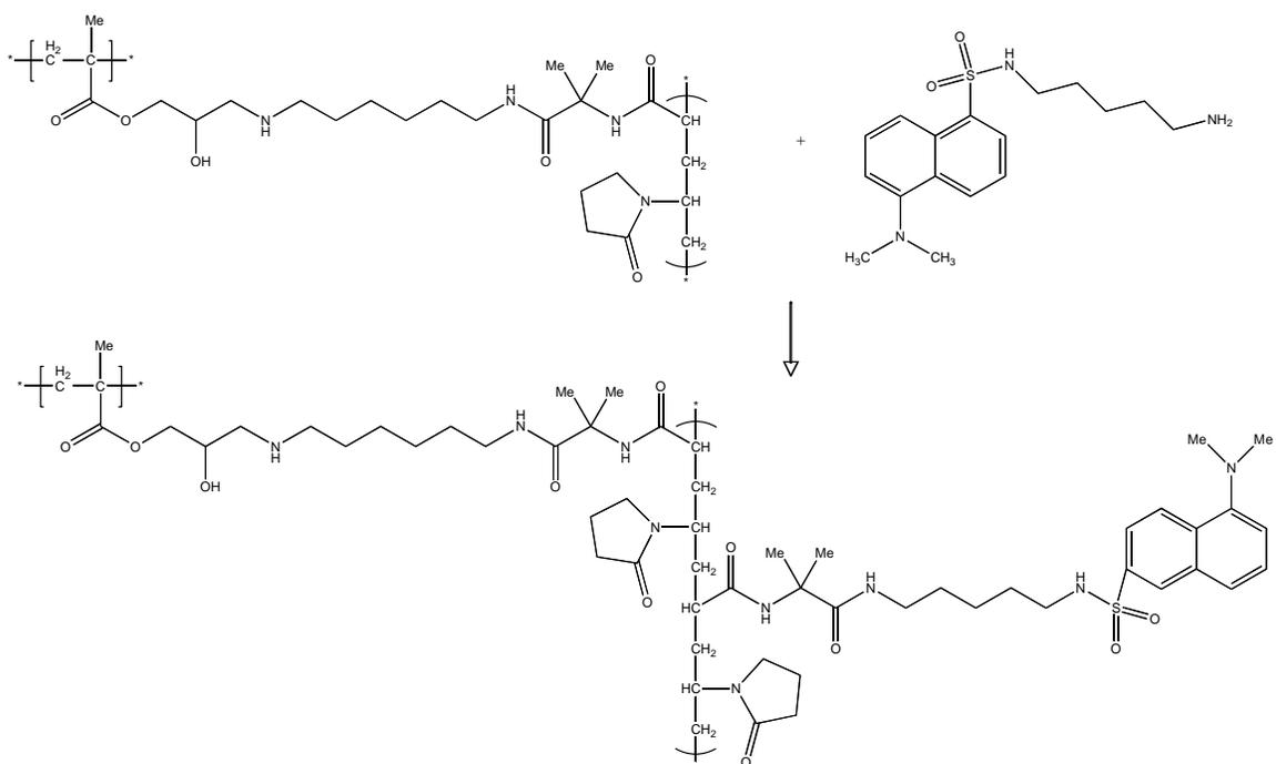
**Scheme 3.3.** The result of the reaction of dansylcadaverine with the PGMA-modified scaffold.
