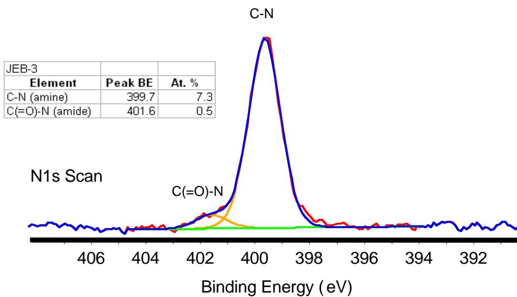
**Figure C.9.** N 1s scan of sample JEB-3 (Amine-modified surface with p(VP-co-VDMA) attachment).
