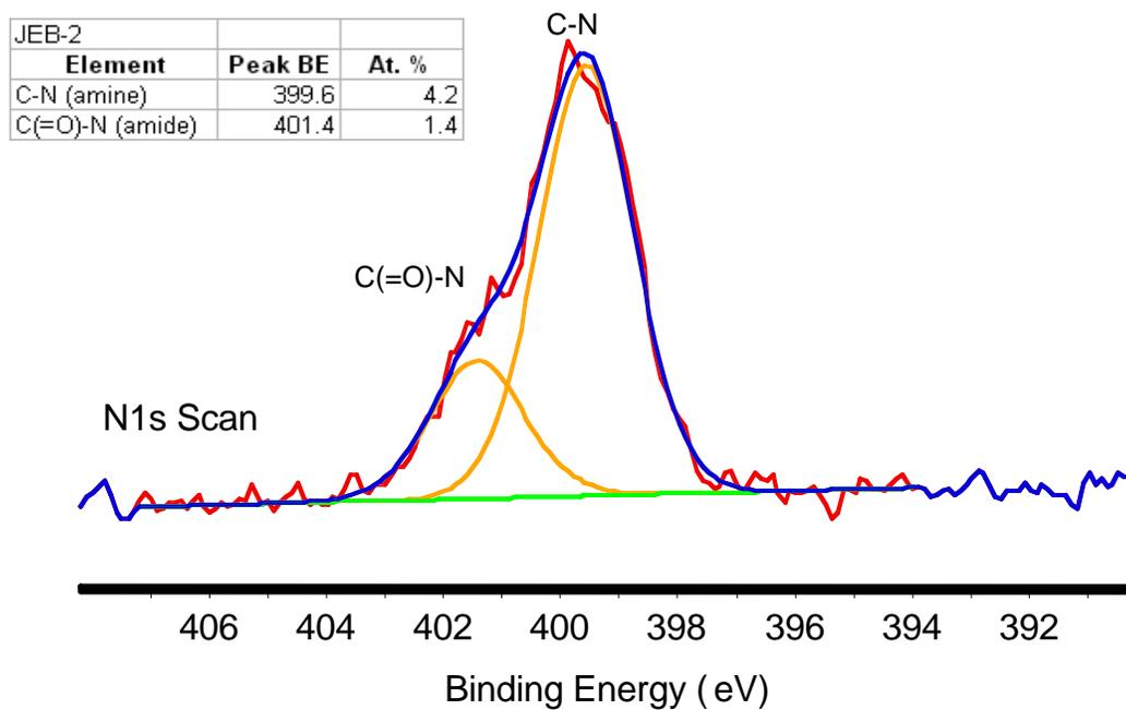
**Figure C.8.** N 1s scan of sample JEB-2 (PGMA with diamine attachment).
