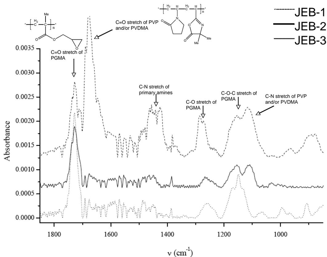
**Figure 3.2.** FTIR spectra showing chemical changes occurring along the progressive steps of the attachment procedure.
