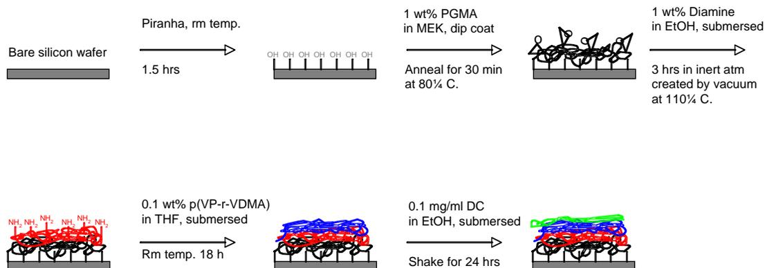
**Scheme 2.1.** Schematic of fluorescent molecule attachment to silicon wafer.
