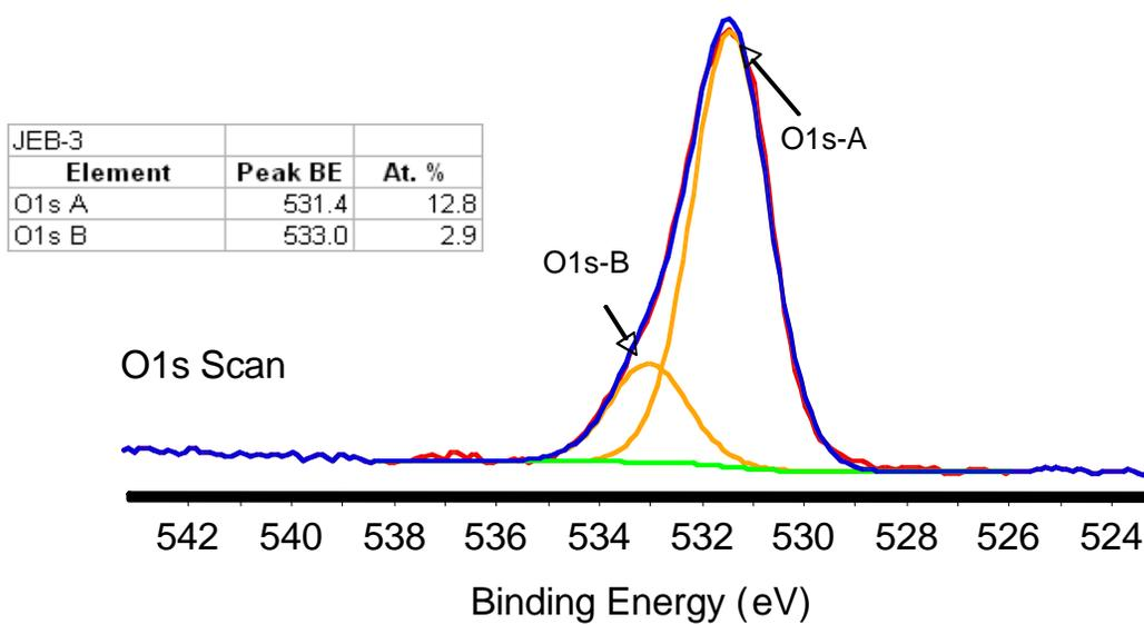
**Figure C.7.** O 1s scan of sample JEB-3 (Amine-modified surface with p(VP-co-VDMA) attachment).
