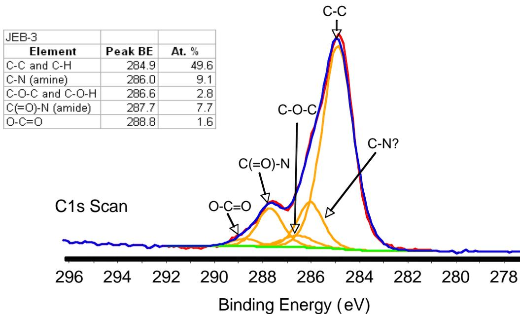
**Figure C.6.** C 1s scan of sample JEB-3 (Amine-modified surface with p(VP-co-VDMA) attachment).
