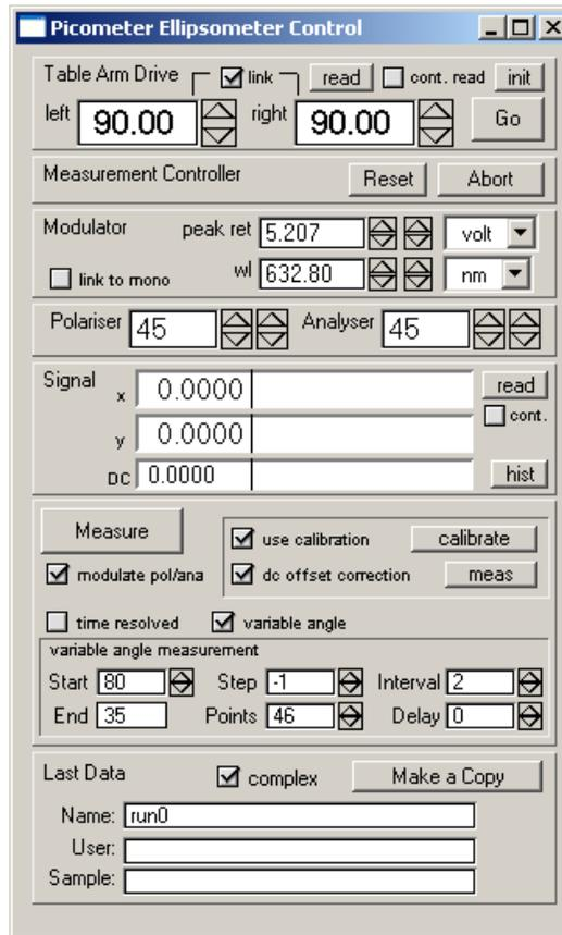
**Figure A.7.** PicoElli Ellipsometer Control panel.
