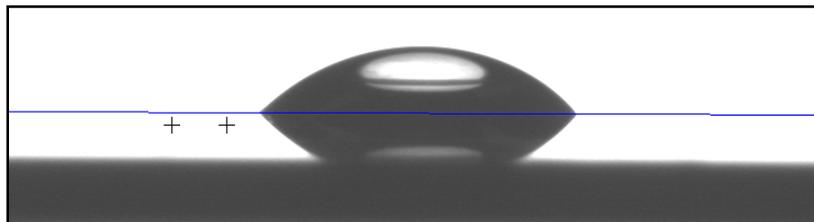
**Figure A.4.** Image a water drop with automatically corrected baseline and “+” for manual baseline correction.
