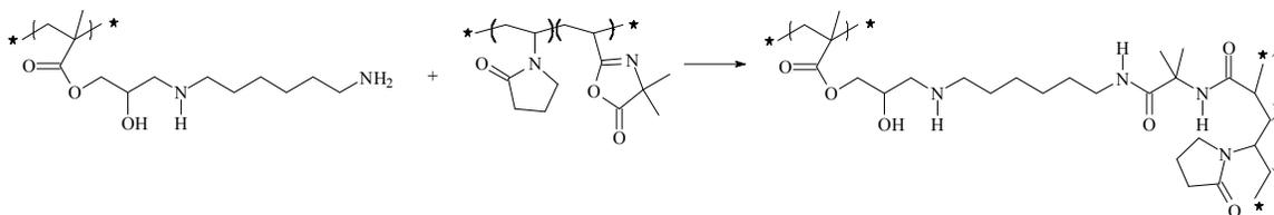
**Scheme 3.2.** Proposed reaction of diamine-modified PGMA with p(VP-co-VDMA).
