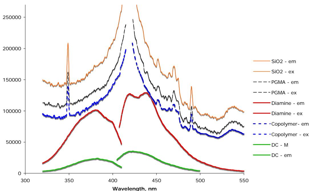
**Figure 3.6.** Fluorometry measurements plotted for each step of the PGMA-modified surface procedure. (Note: “em” designates the emission curves (right side), while “ex” designates the excitation curves (left side).)
