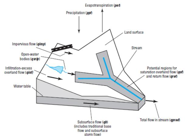
**Figure 2.** Definitions of selected water-source variables from TOPMODEL (modified from Wolock, 1993).
