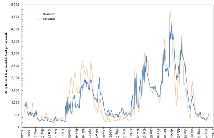
**Figure 3.** Simulated and observed daily mean flow at station 02175000, Edisto River near Givhans, SC, for June 13, 2007, to September 30, 2009.
