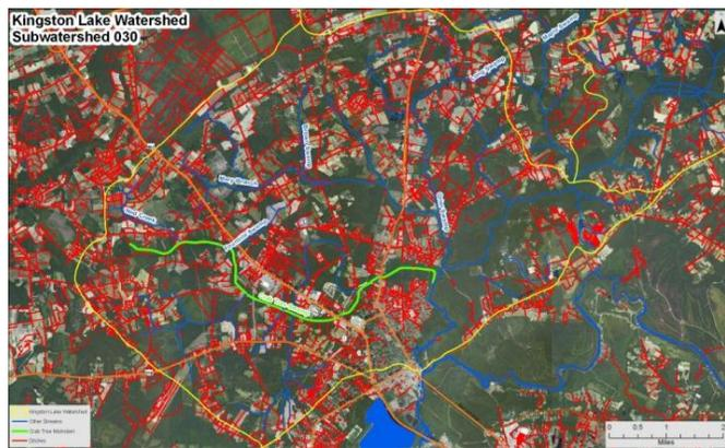
**Figure 4: Hydrological Features in the urban subwatershed of KLW. Manmade features (drainage ditches) are red, natural streamlines are blue, and the channelized portion of Crabtree Swamp, aka Crabtree Canal, is in green.**
