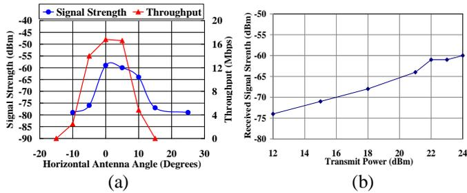
**Figure 4. Long range link's (a) throughput and signal strength at 24 dBm transmit power; (b) signal strength at 7 power levels.**
