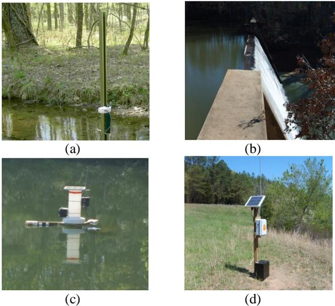
**Figure 2. Local mesh networks connect sensors in forest; (a) inflow Aquarod sensor, (b) outflow sensor, (c) temperature sensor on buoy, and (d) lake side mesh network gateway.**
