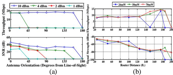
**Figure 5. (a) Throughput and SNR for short range directional link; (b) throughput and signal strength for tree-obstructed link.**
