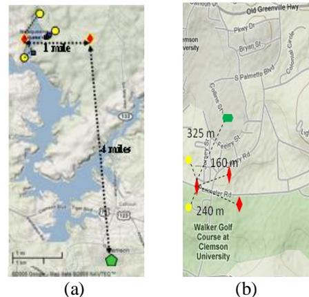
**Figure 1. Network topology at (a) Clemson Forest (b) Hunnicut Creek. Green marks locate the Internet gateways, red marks are transit bridges, and yellow marks show local sensor groups.**
