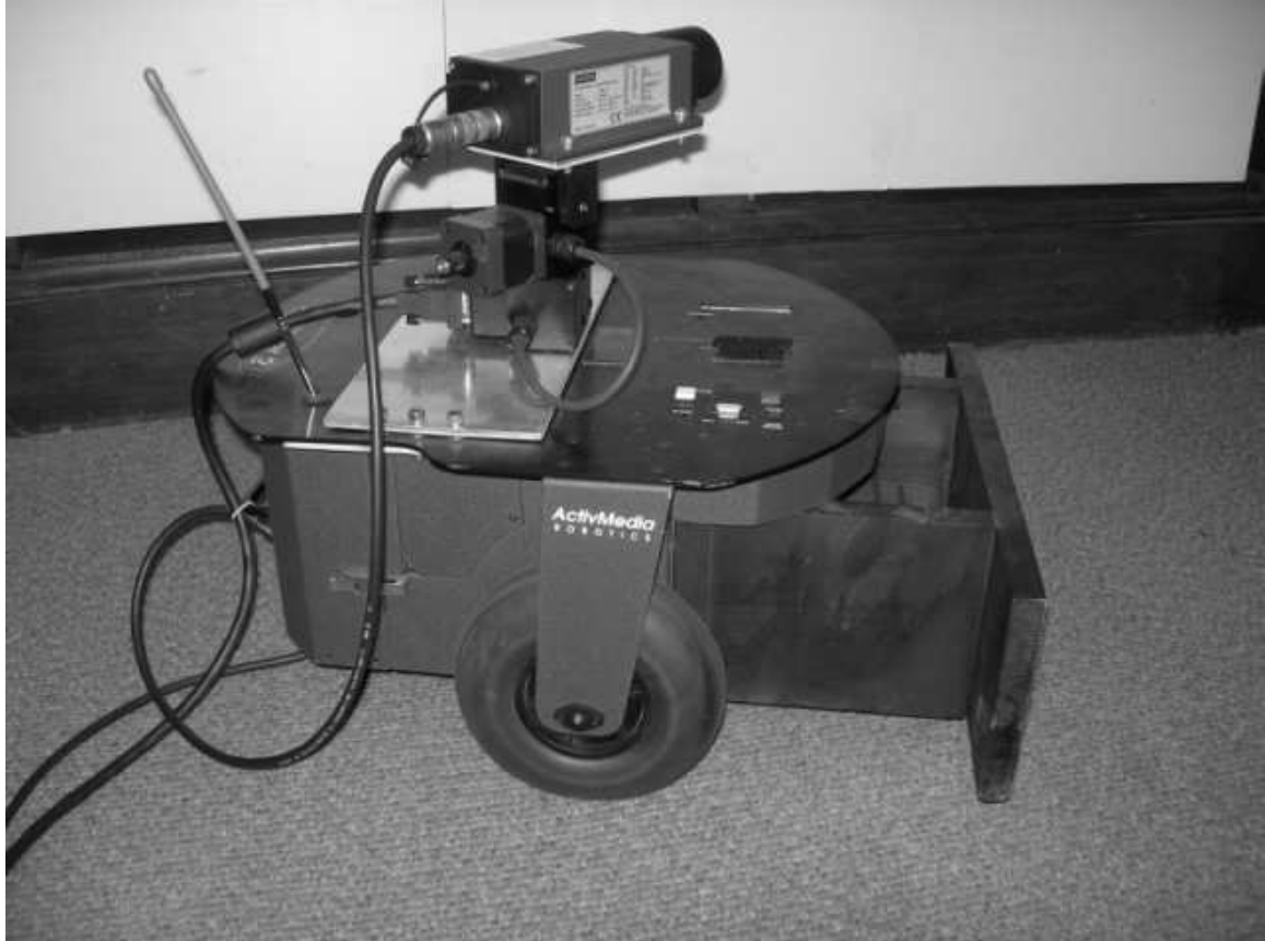
Figure 3.2 Mobile robot with pan-tilt unit and range-finding laser
