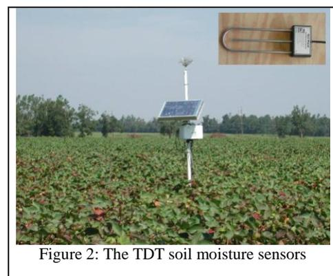
Figure 2: The TDT soil moisture sensors
