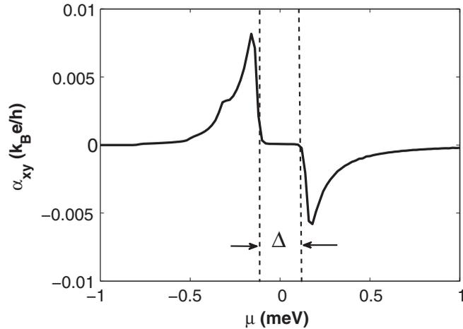
FIG. 3. Anomalous Nernst coefficient versus chemical potential for 2DEG. The dashed lines show the regime of the energy gap  $\Delta$  between the bands. The same parameters have been used as in Fig. 2 with the exception of  $T = 0.1$  K.
