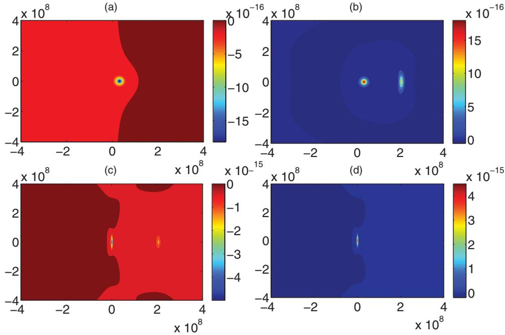
FIG. 6. (Color online) Contour plot of Berry curvature of each band (units of  $m^2$ ) where (a) corresponds to the lowest band and (d) to the highest. The  $y$  and  $x$  axes are  $k_y$  and  $k_x$ , respectively, with units of  $m^{-1}$ . As seen from the denominator of Eq. (10) these functions are sharply peaked at values of  $\mathbf{k}$  near the near-band-degeneracy points.
