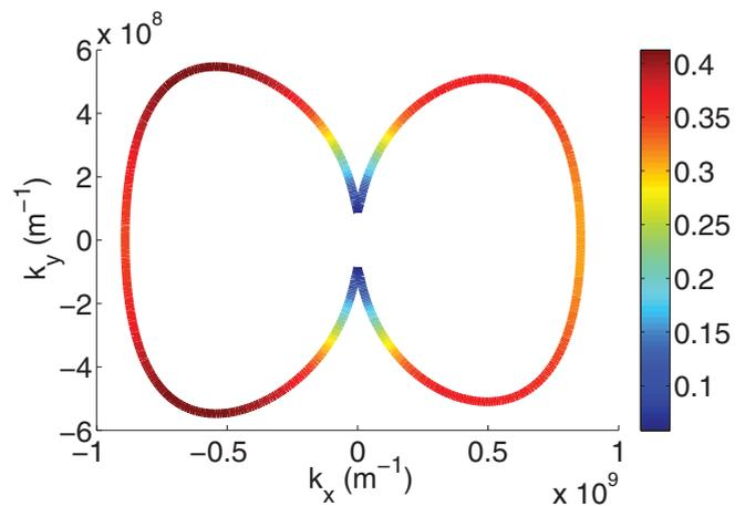
FIG. 5. (Color online) Contour plot of the Fermi surface at  $\mu$  corresponding to the topological regime ( $\mu = -8.5$  meV). Color plot indicates the proportion of light-hole character ( $m_j = \pm 1/2$ ) in the top valence band.
