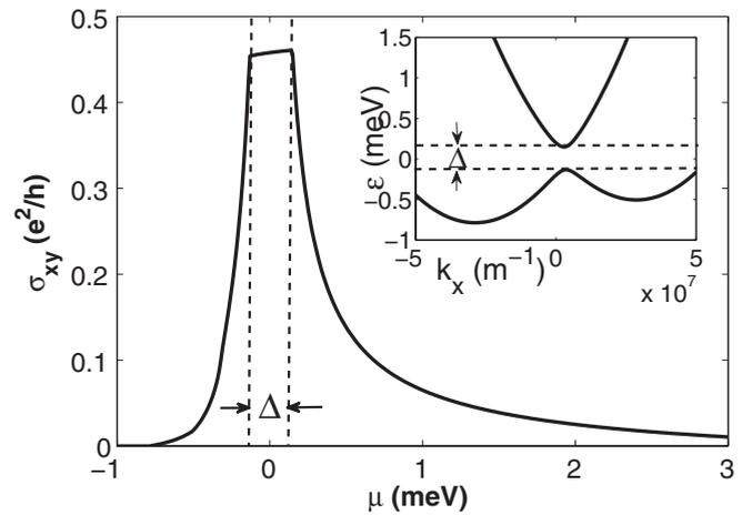
FIG. 2. Anomalous Hall conductivity versus chemical potential  $\mu$  at zero temperature for a two-dimensional electron-doped semiconductor. We have used  $\alpha_R = \alpha_D = 4.74 \times 10^4$  m/s,  $m^* = .067m_e$ , and  $h_y = 0.2$  meV. The electronic band structure versus  $k_x$  is shown in the inset along with the minimum energy gap  $\Delta$  indicated by the dashed lines.
