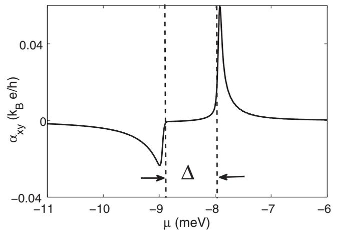
FIG. 8. Plot of the anomalous Nernst coefficient for the [110]-grown hole-doped quantum well near the topological regime of the chemical potential. The topological regime of  $\mu$  is characterized by a plateau of the anomalous Nernst coefficient (at vanishing values) flanked by two peaks of opposite signs as in the case of the electron-doped semiconductors. The parameters used are the same as in Fig. 4 except that  $T = 0.1$  K.
