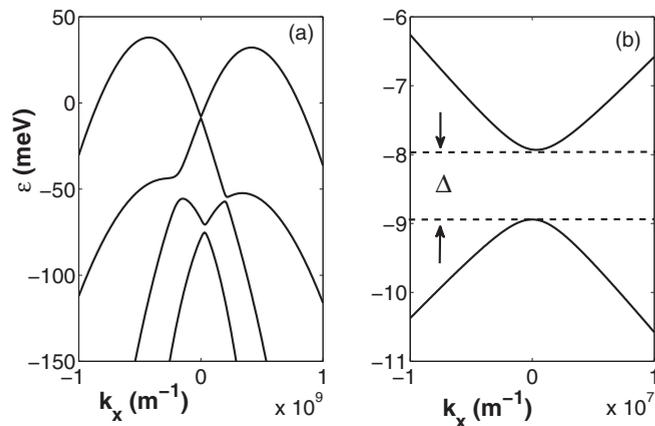
FIG. 4. (a) Band structure of the 2DHG in the  $k_x$  direction for  $k_y = 0$ . (b) Energy gap at origin between lower bands. Here we have used  $\alpha_R = \alpha_D = 2 \times 10^5$  m/s,  $h_y = 5$  meV,  $\gamma_1 = 6.92$ ,  $\gamma_2 = 2.1$ ,  $\gamma_3 = 2.9$ , and  $a = 8$  nm which are chosen for GaAs.
