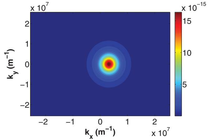
FIG. 1. (Color online) Contour plot of the Berry curvature  $\boldsymbol{\Omega}_{-}$  in the lower band of electron-doped semiconductors. The Berry curvature is sharply peaked at a finite value of  $k_x$  near the band-degeneracy point in the absence of the Dresselhaus coupling.
