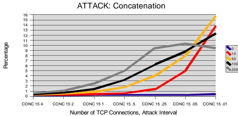
**Figure 5.26.** Percentage of packets transmitted via concatenation for 15 TCP connections, number of nodes attacked range from zero to 200, attack rate interval range from 4 to .01 seconds. As the attack rate interval approaches .01 seconds, the percentage of packets sent via concatenation increases.
