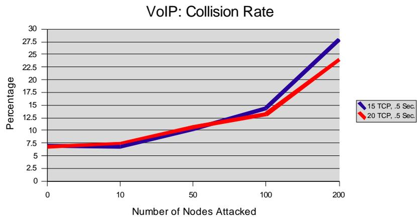
**Figure 5.6.3.** Collision rate (y-axis) for VoIP cable modem, 400 cable modems, .5 second attack rate interval, range of nodes attacked zero to 200 (x-axis). Over 80 percent change in rate from 100 to 200 nodes attacked, 15 TCP connections.
