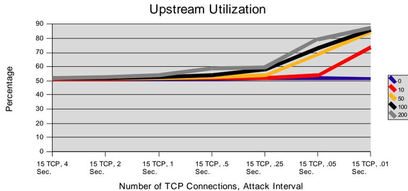
**Figure 5.18.** Upstream utilization for 15 TCP connections, range of nodes attacked from zero to 200, and an attack rate interval range of 4 seconds to .01 seconds. As the attack rate interval was increased (approached 4 seconds), upstream utilization decreased. As the attack rate interval was decreased (approaches .01 seconds), the upstream utilization increased.
