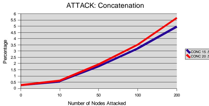
**Figure 5.11.** The percentage of packets sent via concatenation as the number of nodes attacked increases. 400 cable modems, .5 second attack interval, range of nodes attacked from zero to 200. The percentage of packets sent via concatenation increased, as expected, with the number of nodes attacked increased.
