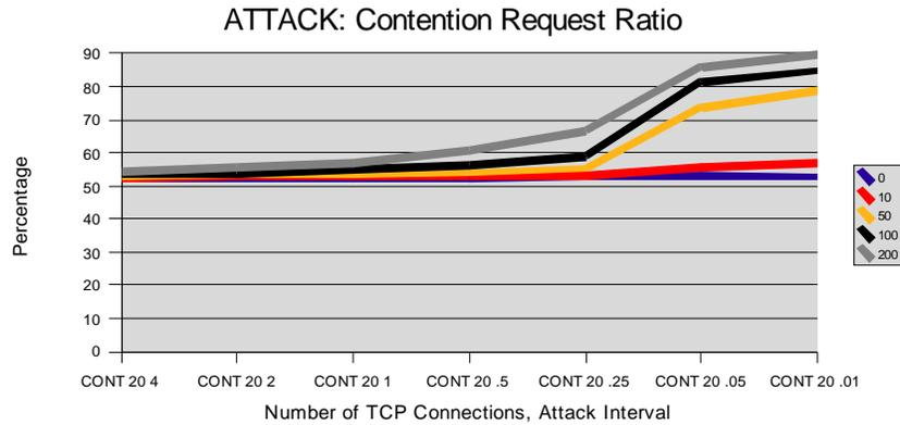
**Figure 5.23.** Contention request ratio for 20 TCP connections, number of nodes attacked range from zero to 200, attack rate interval range from 4 to .01 seconds. As the interval between attack packets decreases, the number of contention requests required to transmit a packet increases.
