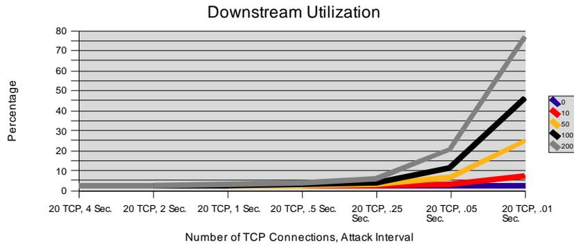
**Figure 5.17.** Downstream utilization for 20 TCP connections, range of nodes attacked from zero to 200, and an attack rate interval range of 4 seconds to .01 seconds. As the attack rate interval was increased (approached 4 seconds), downstream utilization decreased. As the attack rate interval was decreased (approaches .01 seconds), the downstream utilization increased.
