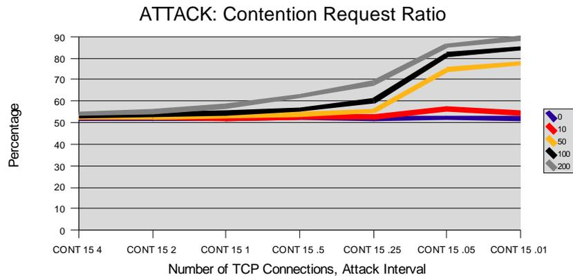
**Figure 5.22.** Contention request ratio for 15 TCP connections, number of nodes attacked range from zero to 200, attack rate interval range from 4 to .01 seconds. As the interval between attack packets decreases, the number of contention requests required to transmit a packet increases.
