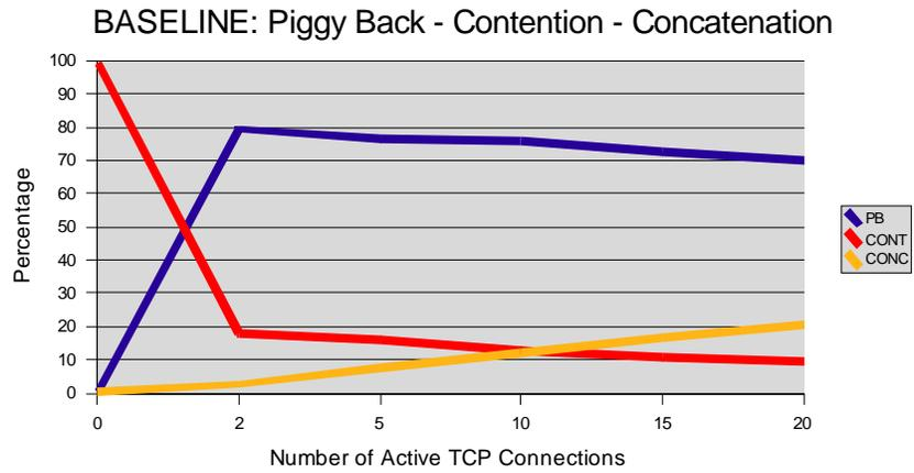
**Figure 5.3.** Percentage of packets sent via piggybacking, contention request, and concatenation observed during simulation of baseline configuration. 400 cable modems, range of active TCP connections a follows: 0, 2, 5, 10, 15, and 20.
