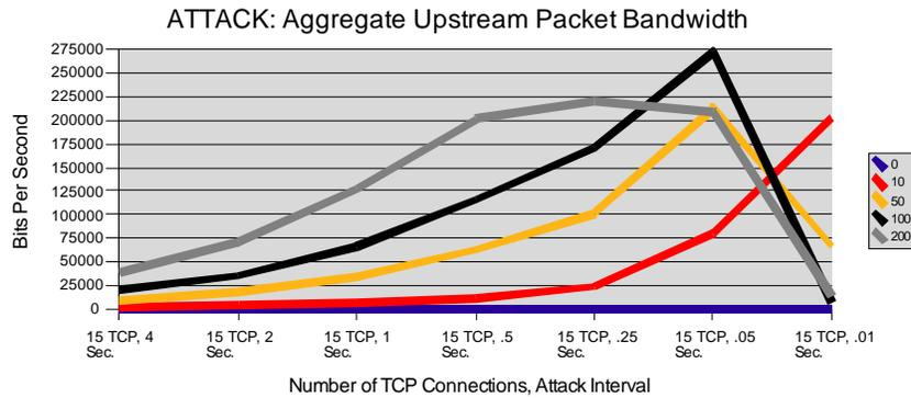
**Figure 5.14.** The aggregate upstream attack packet bandwidth in bits per second (y-axis) as the attack rate interval is decreased from 4 seconds to .01 seconds (x-axis). As the attack rate interval increases (approaches 4 seconds), upstream bandwidth consumes decreases. As the attack rate interval decreases (approaches .01 seconds), Upstream bandwidth consumed increases.
