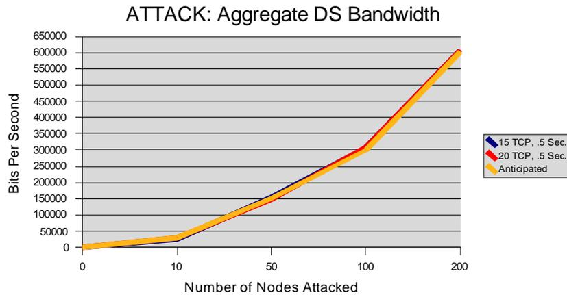
**Figure 5.4.** Aggregate downstream attack packet bandwidth, 400 cable modems, .5 second attack interval, across the number of nodes attacked (x-axis) in bits per second (y-axis). Also graphed is the anticipated bandwidth given the rate of attack.
