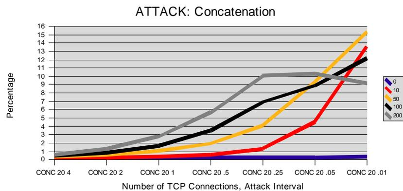
**Figure 5.27.** Percentage of packets transmitted via concatenation for 20 TCP connections, number of nodes attacked range from zero to 200, attack rate interval range from 4 to .01 seconds. As the attack rate interval approaches .01 seconds, the percentage of packets sent via concatenation increases.
