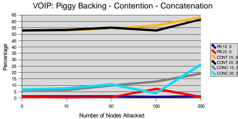
**Figure 5.8.1.** Percentage of VoIP packets sent via piggybacking, contention requests without concatenation, and with concatenation for 400 cable modems, .5 second attack interval, number of nodes attacked range from zero to 200. Compared to attack packet behavior, VoIP packets utilize less piggybacking and more concatenation.
