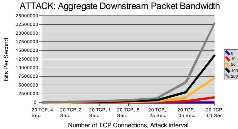
**Figure 5.13.** The aggregate downstream attack packet bandwidth in bits per second (y-axis) as the attack rate interval is decreased from 4 seconds to .01 seconds (x-axis). As the attack rate interval increases (approaches 4 seconds), downstream bandwidth consumed decreases. As the attack rate interval decreases (approaches .01 seconds), downstream bandwidth consumed increases.
