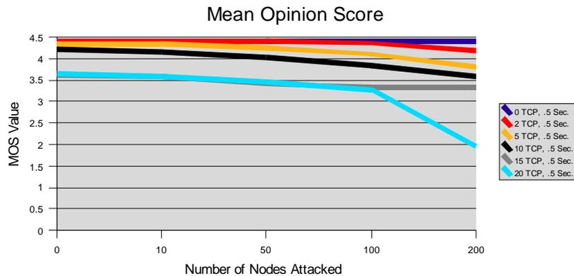
**Figure 5.6.1.** MOS value observed with 400 cable modems, .5 second attack interval, number of nodes attacked range from zero to 200. First MOS value observed below the thesis benchmark of 3.0 is at 200 nodes attacked with 20 TCP connections active (light blue).
