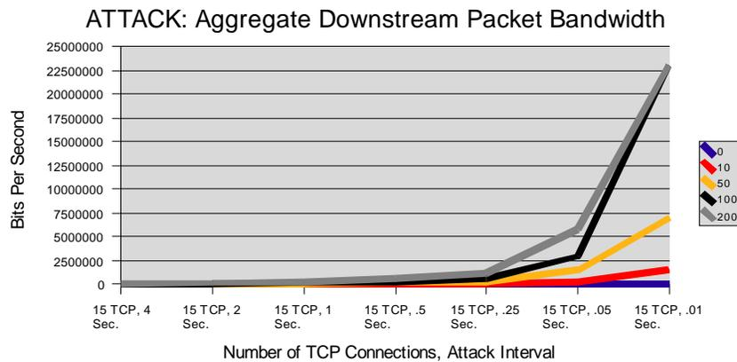
**Figure 5.12.** The aggregate downstream attack packet bandwidth in bits per second (y-axis) as the attack rate interval is decreased from 4 seconds to .01 seconds (x-axis). As the attack rate interval increases (approaches 4 seconds), downstream bandwidth consumed decreases. As the attack rate interval decreases (approaches .01 seconds), downstream bandwidth consumed increases.
