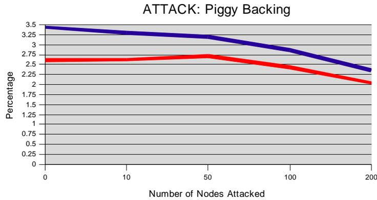
**Figure 5.9.** Percentage of packets sent via piggybacking as the number of nodes attacked increased. 400 cable modems, .5 second attack interval, range of nodes attacked from zero to 200. The number of packets sent via piggybacking decreased as the number of nodes attacked was increased.
