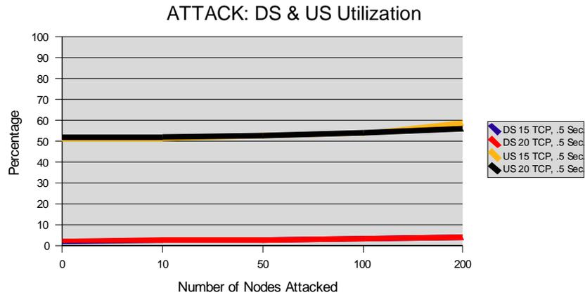
**Figure 5.7.** Downstream and upstream utilization for 400 cable modems, .5 second attack interval, number of nodes attacked range from zero to 200. Significance observed is the extremely low percentage of the downstream channel required to achieve the DoS attack objective, as well as, the impact on the upstream channel.
