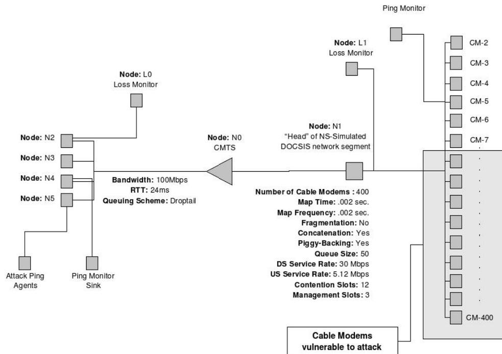
**Figure 4.1.** Network map and configuration settings used as the test network for this thesis. On the left side of the figure is the WAN-side nodes (Internet-residing nodes). On the right side are cable modems belonging to the private, DOCSIS-based network.
