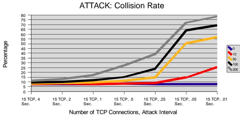
**Figure 5.20.** Collision rate (y-axis) for 15 TCP connections, number of nodes attacked range from zero to 200, and attack rate interval range of 4 to .01 seconds. Decrease in attack rate interval results in an increase in collision rate.
