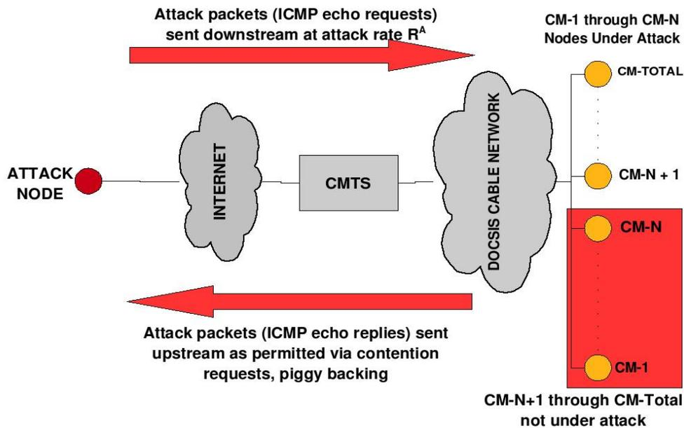
**Figure 3.1.** Graphical depiction of simulated network general layout. The attack node is located on any network outside of the DOCSIS network. The nodes labeled CM-1 through CM-N do not support any management or monitoring services and are “vulnerable” to the DoS attack. Nodes CM-N+1 to CM-Total support management and monitoring services (TCP traffic replicating varying network nodes, loss monitor, VoIP monitor).
