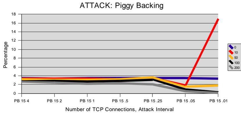
**Figure 5.24.** Percentage of packets transmitted via piggybacking for 15 TCP connections, number of nodes attacked range from zero to 200, attack rate interval range from 4 to .01 seconds. As attack rate interval decreases from 4 to .01 seconds, percentage of packets sent via piggybacking decreases.
