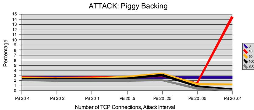
**Figure 5.25.** Percentage of packets transmitted via piggybacking for 20 TCP connections, number of nodes attacked range from zero to 200, attack rate interval range from 4 to .01 seconds. As attack rate interval decreases from 4 to .01 seconds, percentage of packets sent via piggybacking decreases.
