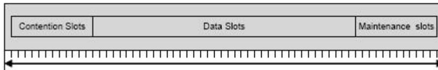
**Figure 2.2.** DOCSIS bandwidth allocation map (MAP). The contention slots are used by the cable modems to request access to the upstream channel from the cable modem termination system. The data slots are used after access has been granted to a cable modem to transmit data. The maintenance slots are used for initialization and synchronization when a cable modem powers on.
