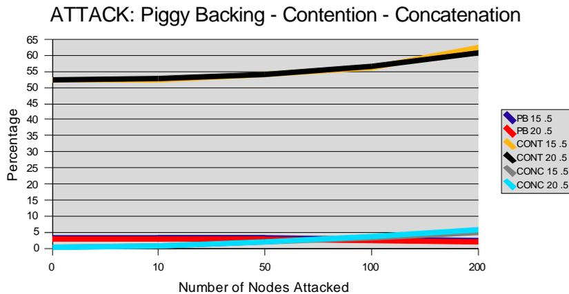
**Figure 5.8.** Percentage of packets sent via piggybacking, contention requests without concatenation, and with concatenation for 400 cable modems, .5 second attack interval, number of nodes attacked range from zero to 200. The observed behavior was in-line with what was expected, as the number of nodes attacked increased, the ratio of contention requests to total packets sent and packets sent via concatenation increased while the number of packets sent via piggybacking decreased.
