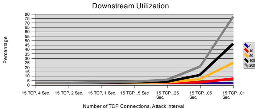
**Figure 5.16.** Downstream utilization for 15 TCP connections, range of nodes attacked from zero to 200, and an attack rate interval range of 4 seconds to .01 seconds. As the attack rate interval was increased (approached 4 seconds), downstream utilization decreased. As the attack rate interval was decreased (approaches .01 seconds), the downstream utilization increased.
