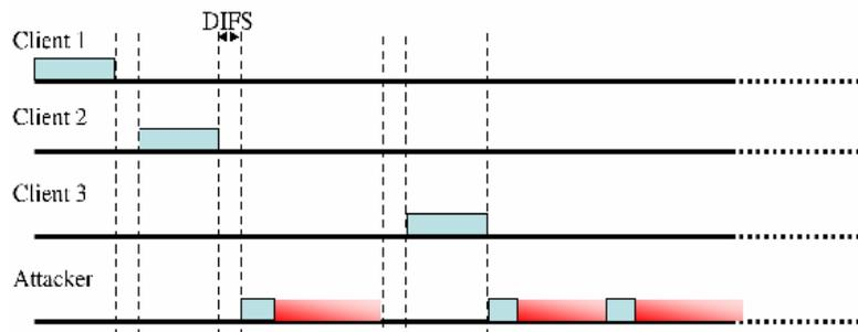
**Figure 2.4.** Graphical depiction of the virtual carrier-sense attack in action. The gradient portion of the attacker's frame indicates time reserved by the duration field although no data is actually sent. Continually sending the attack frames back to back prevents other nodes from sending legitimate frames [Bellardo, 2003].
