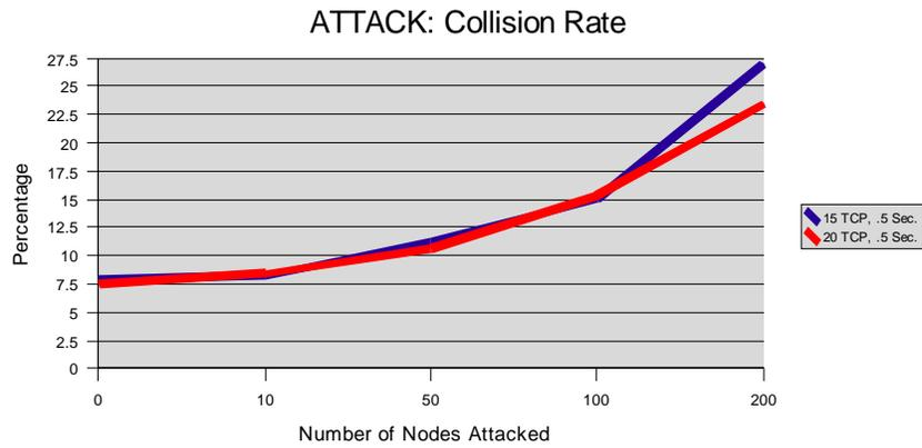
**Figure 5.6.2.** Collision rate (y-axis) for cable modems under attack, 400 cable modems, .5 second attack rate interval, range of nodes attacked zero to 200 (x-axis). Over 80 percent change in rate from 100 to 200 nodes attacked, 15 TCP connections.
