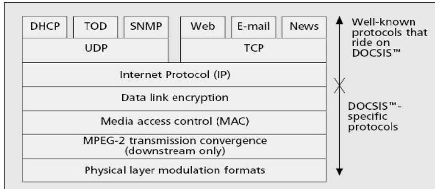
**Figure 2.1.** The DOCSIS cable modem protocol stack. The physical layer is where modulation of the signal occurs. The cable modem termination system adds framing using MPEG-2 transmission convergence protocol enabling multiple services to be sent on the same channel. The MAC layer is where access to the upstream path is managed.
