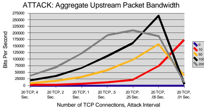
**Figure 5.15.** The aggregate upstream attack packet bandwidth in bits per second (y-axis) as the attack rate interval is decreased from 4 seconds to .01 seconds (x-axis). As the attack rate interval increases (approaches 4 seconds), upstream bandwidth consumes decreases. As the attack rate interval decreases (approaches .01 seconds), Upstream bandwidth consumed increases.
