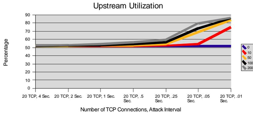
**Figure 5.19.** Upstream utilization for 20 TCP connections, range of nodes attacked from zero to 200, and an attack rate interval range of 4 seconds to .01 seconds. As the attack rate interval was increased (approached 4 seconds), upstream utilization decreased. As the attack rate interval was decreased (approaches .01 seconds), the upstream utilization increased.
