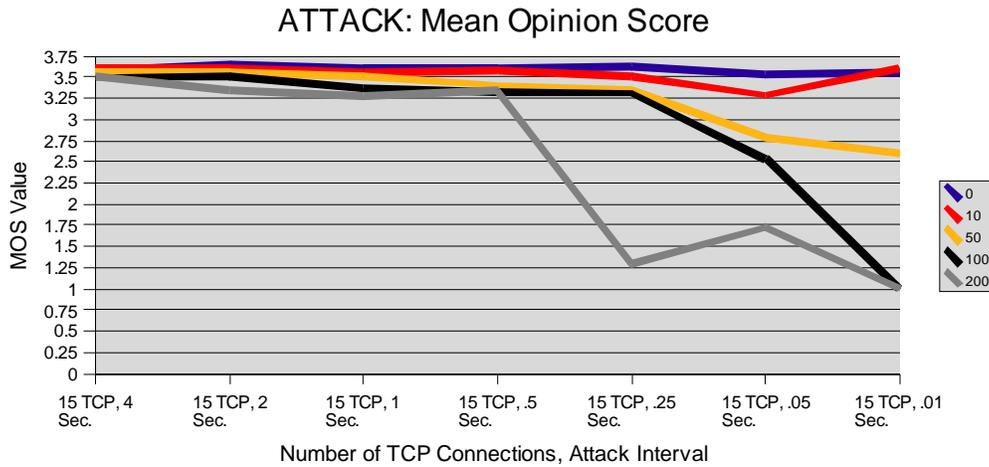
**Figure 5.11.1.** Mean Opinion Score (y-axis) for 15 TCP connections, range of nodes attacked from zero to 200, and a attack rate interval range from 4 to .01 seconds (x-axis). An MOS value less than the threshold value of 3.0 is first observed at 200 nodes attacked and an attack rate interval of .25 seconds. A sub-3.0 MOS value is observed at 50, 100, and 200 nodes attacked with an attack rate interval of .05 and .01 seconds.
