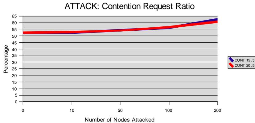
**Figure 5.10.** The ratio of contention requests to total packets sent as the number of nodes attacked increased. 400 cable modems, .5 second attack interval, range of nodes attacked from zero to 200. The ratio of contention requests to total packets sent increased, as expected, as the number of nodes attacked increased.
