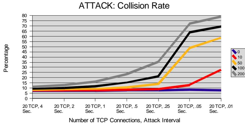
**Figure 5.21.** Collision rate (y-axis) for 20 TCP connections, number of nodes attacked range from zero to 200, and attack rate interval range of 4 to .01 seconds. Decrease in attack rate interval results in an increase in collision rate.
