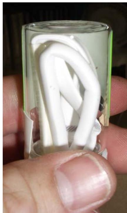
**Figure 3. The GORE™ Module after it was retrieved from a borehole and prior to being shipped to the laboratory for analysis.**
