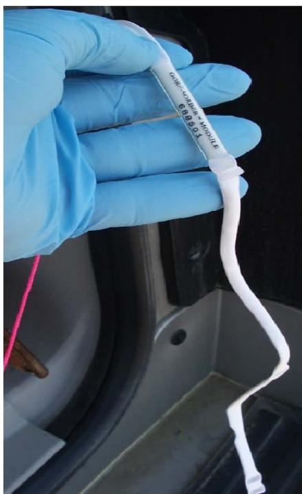
**Figure 2. The GORE™ Module ready to be installed in a shallow borehole in the field.**
