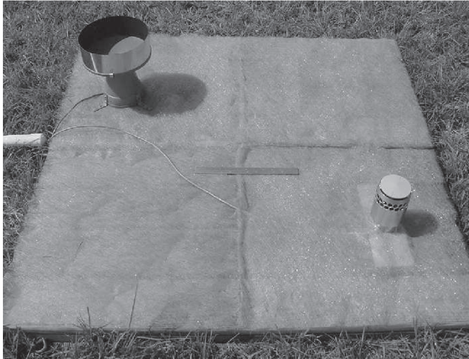
Figure 1: Joss-Waldvogel type momentum disdrometer shown with tipping-bucket rain gage, installed for data collection. Fiberglass material was attached to the installation platform around the instruments to reduce spatter from drops that did not hit the instruments
