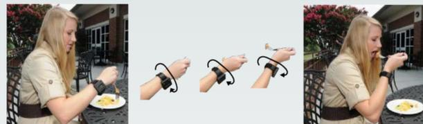
Figure 1. Wrist-roll measured by the Bite Counter.
