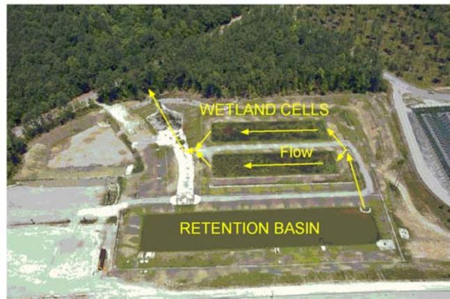
Figure 2. Layout and water flow path through CWTS for H-02 outfall.
