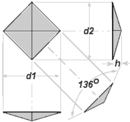
**Figure 4.3:** Illustration of the indentation made from the micro-hardness indenter. The  $d1$  and  $d2$  dimensions were used with the Vicker's hardness method to establish a hardness value of the bone (Richard E. Thacker, 2004).
