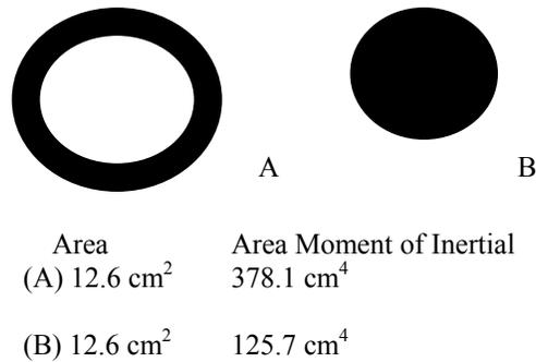
**Figure 1.2:** Representation of a tube and a rod, which respective moment of inertias. (A) Representation of tub (bone), (B) Representation of a regular rod. The areas of these figures are represented by the black and are assumed to be equal. These two figures show the difference in arrangement of bone within the long bones. It has the material moved to the outer areas that carry more load and no material is being wasted in the center.
