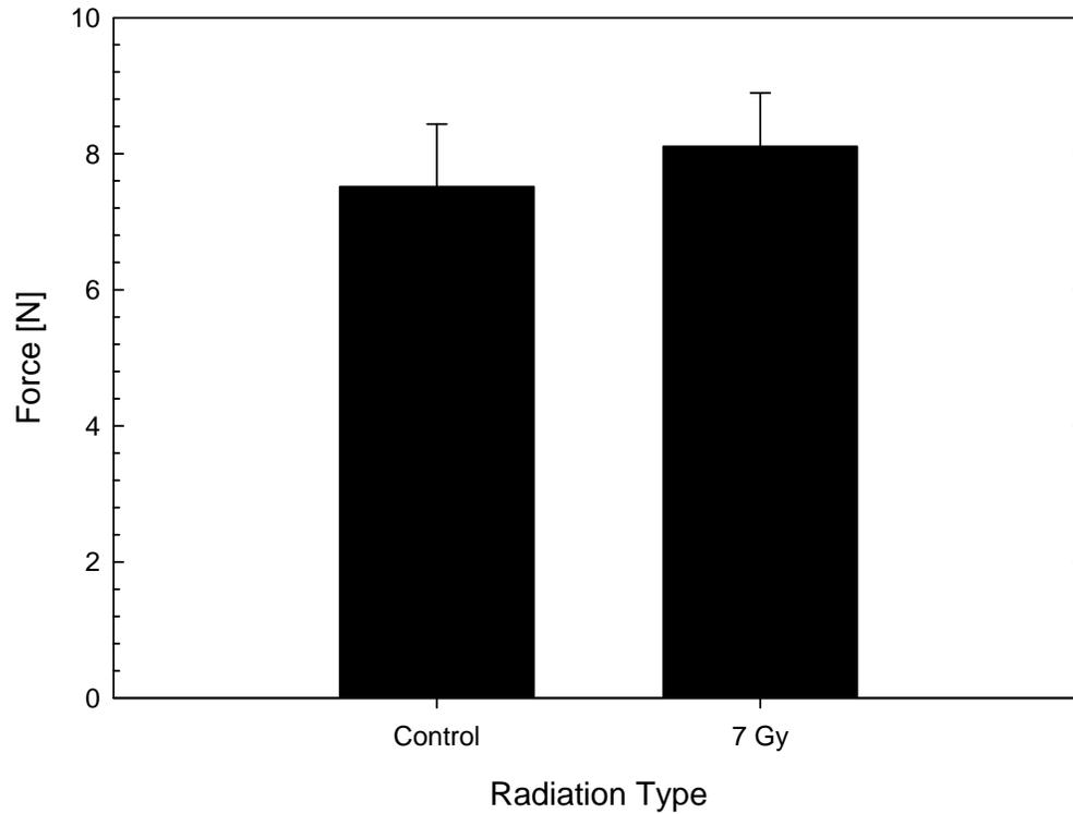
**Figure 4.6:** Fracture Force of High-Dose bones, error bars using standard error of the mean
