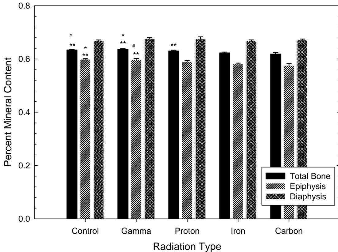
**Figure 3.4:** Percent mineral content of Multi-Type study, error bars using standard error of the mean. The epiphysis and diaphysis is broken up into individual bars with and additional bar for the whole femur. \* Denotes significant difference from Iron, \*\* Denotes significant difference from Carbon, # Denotes trend with Iron.
