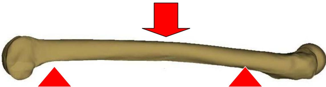
**Figure 4.1:** Illustration of a three point bending technique used in the mechanical testing of these femora. The bone is in the correct anatomical position for testing.
