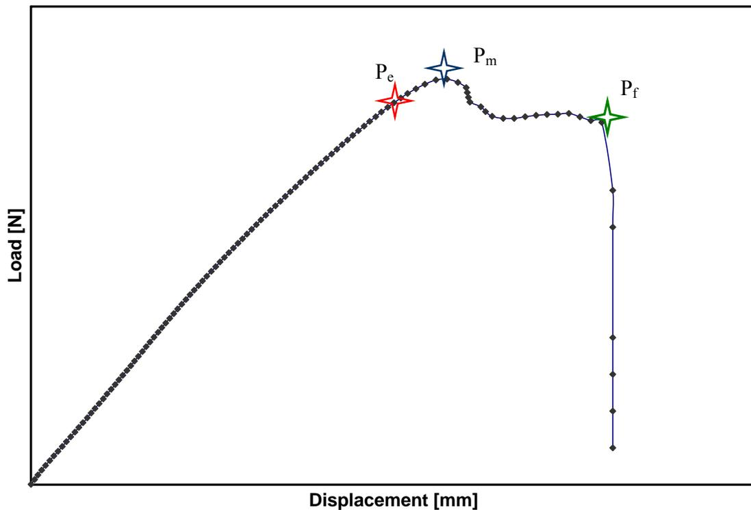
**Figure 3.1:** This figure represents an idealized load versus displacement curve for the output of the mechanical data measure. The points mark the places on the curve where mechanical values were determined.
