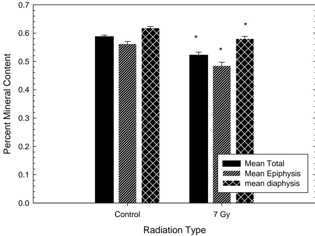
**Figure 4.4:** Percent mineral content of High-Dose femora, error bars using standard error of the mean. \* Denotes statistically significant difference from control. All parts of the irradiated group are different from the control group.
