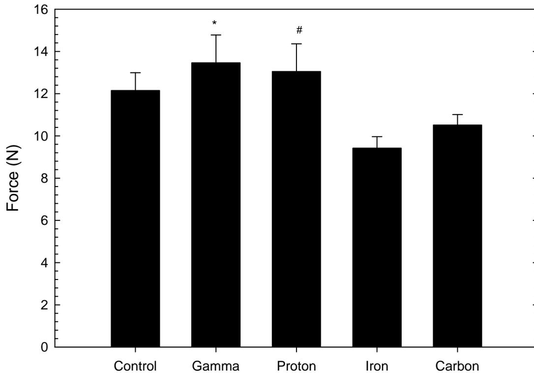
**Figure 3.5:** Fracture force of Multi-Type, Gamma was found to have a significantly greater fracture force than iron,  $P=0.034$ . Additionally, with the proton group a trend of a higher fracture force was seen when compared to iron,  $P=0.07$ . \* Denotes difference from iron, error bars using standard error of the mean. # Denotes a trend from iron.
