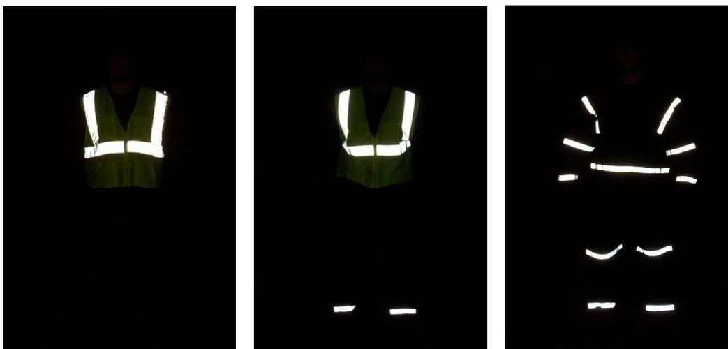
Figure 3. Frontal view of the three clothing configurations: Vest only, Vest + Ankles, and Full Biomotion.
