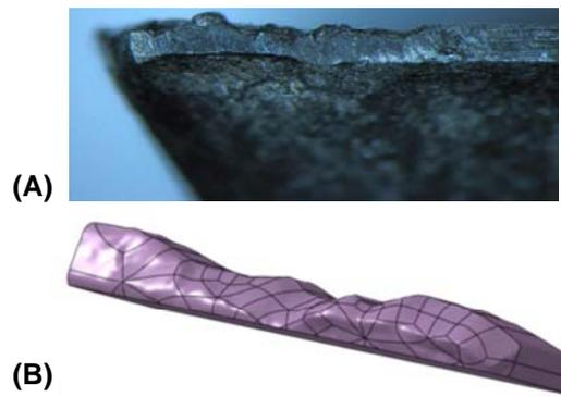
**FIGURE 9 - INSERT AFTER A CUTTING LENGTH OF 154.8 MM, A) MICROSCOPE IMAGE AND B) SOLID MODEL FOR VOLUMETRIC COMPARISON**
