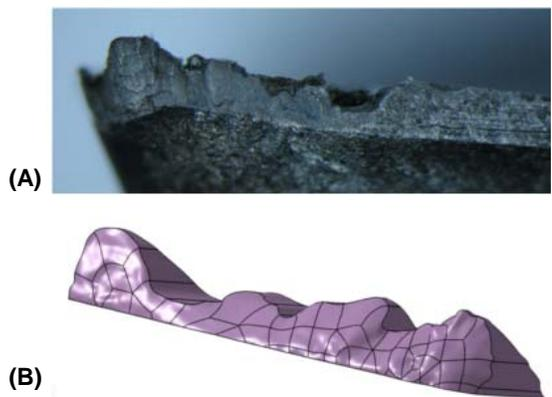
**FIGURE 10 - INSERT AFTER A CUTTING LENGTH OF 309.6 MM, A) MICROSCOPE IMAGE AND B) SOLID MODEL USED FOR VOLUMETRIC COMPARISON**
