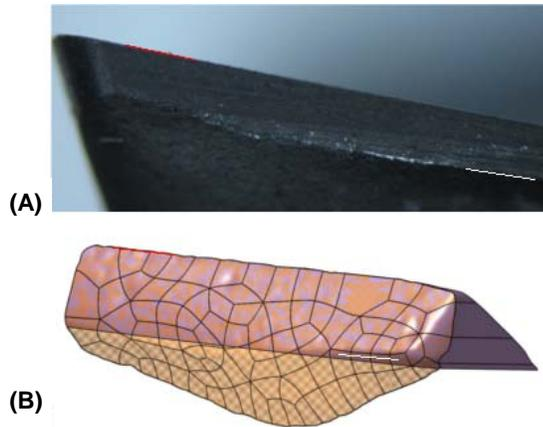
**FIGURE 7 - UNWORN INSERTS, A) MICROSCOPE IMAGE AND B) SOLID MODEL FOR MEASUREMENTS ALONG WITH REFERENCE SURFACE**
