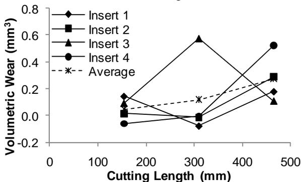
FIGURE 13 - VOLUMETRIC WEAR PLOTS FOR INDIVIDUAL INSERTS IN EXPERIMENT 2
