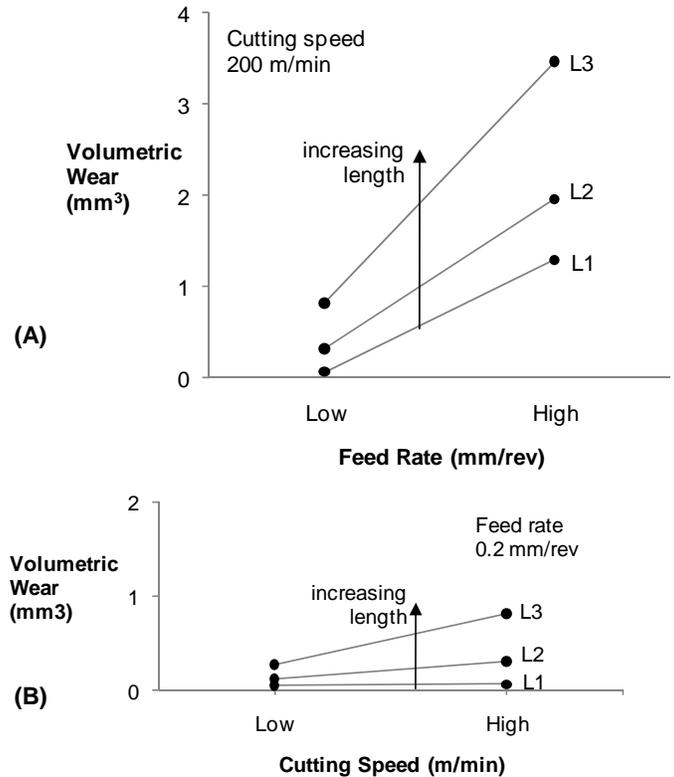
**FIGURE 12 – A) AVERAGE VOLUMETRIC WEAR VS FEED FOR EXPERIMENTS 1-3 B) AVERAGE VOLUMETRIC WEAR VS SPEED FOR EXPERIMENTS 1-3**
