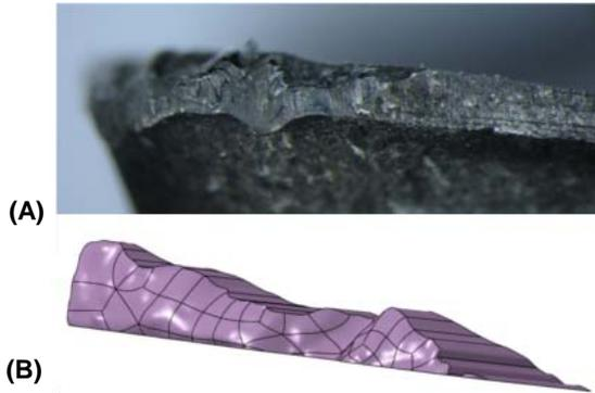
**FIGURE 11 - INSERT AFTER A CUTTING LENGTH OF 464.4 MM, A) MICROSCOPE IMAGE AND B) SOLID MODEL USED FOR VOLUMETRIC COMPARISON**
