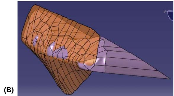
**FIGURE 8 - MATCHING PROCESS, A) SURFACE MATCHING BETWEEN WORN AND UNWORN SURFACES AND B) SOLID MODEL OF WORN INSERT WITH UNWORN REFERENCE SURFACE**
