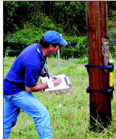
**Figure 2.** Water-level sensor device attached to power pole.
