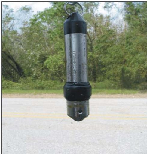
**Figure 1.** Sensor used to collect water-level and barometric-pressure data.
