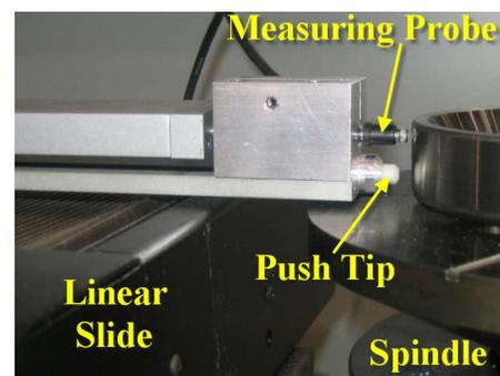
Figure 1 - Centering System Components
