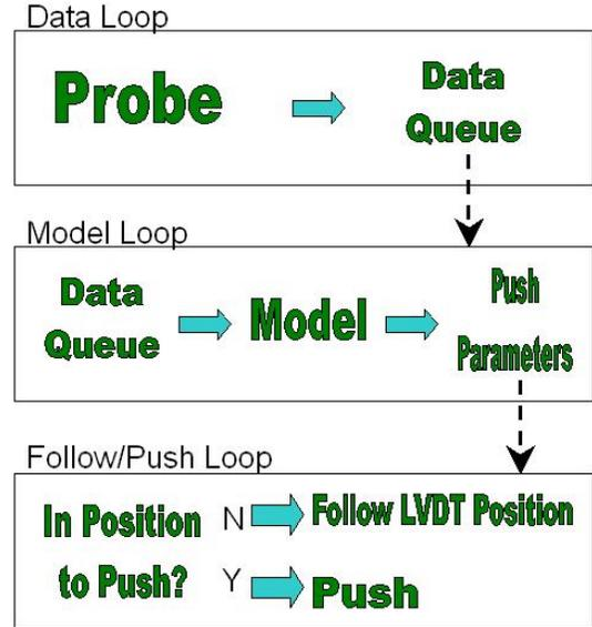
Figure 2 - Algorithm Parallel Loop Structure (Communication Loop not shown)
