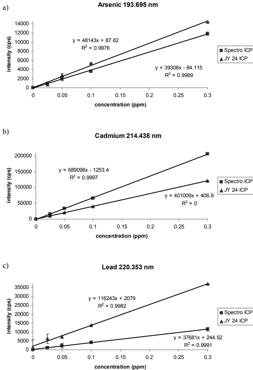
Figure 2.1: Calibration functions of a) arsenic, b) cadmium, and c) lead on the JY 24 ICP-AES and the Spectro ICP-AES instruments.
