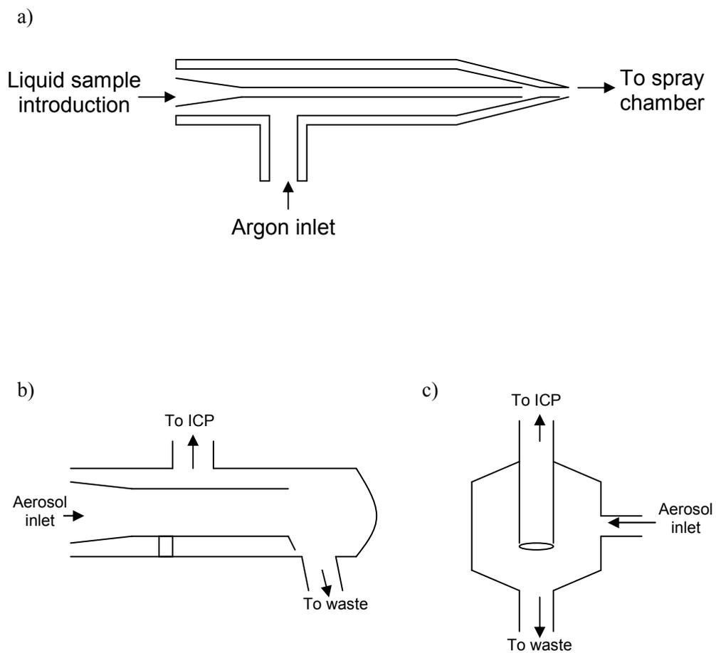
Figure 1.3: a) Schematic of a pneumatic nebulizer. b) Schematic of a Scott-type spray chamber and c) cyclonic spray chamber.
