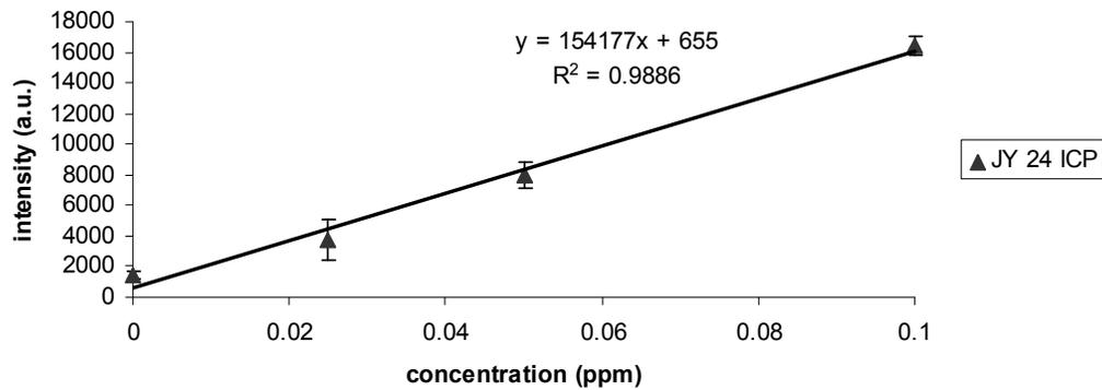
Figure 2.3: Standard addition functions for a) cadmium and b) lead in SRM 3243 in preliminary validation experiments on the JY 24 ICP.
