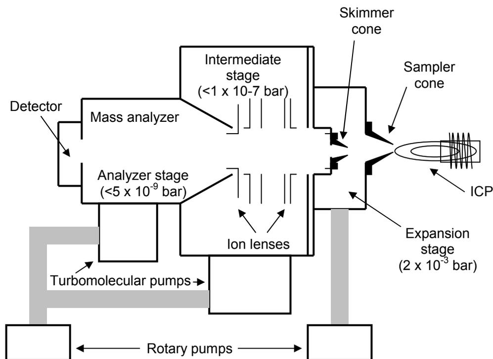
Figure 1.6: Generalized schematic of an ICP-MS instrument.
