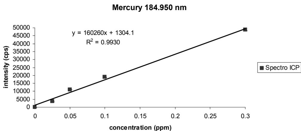
Figure 2.2: Calibration functions for mercury on the a) JY 24 ICP-AES, with the function forced through zero, and on the b) Spectro ICP-AES instruments.
