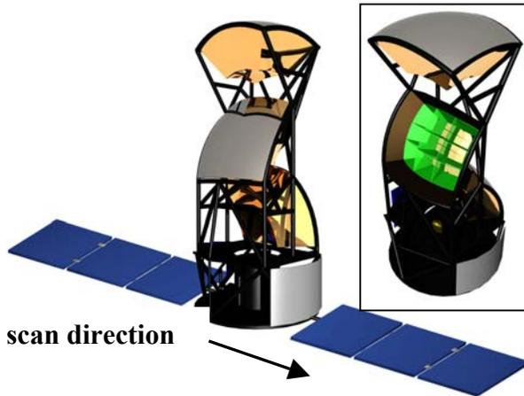
**FIGURE 1.** a) *EXIST* telescopes (3) on spacecraft, zenith pointed along orbital scan direction, b) cutaway view showing imaging CZT detector arrays and active collimator.
