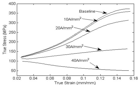
FIGURE 4. FLOW STRESS OF EAM MAGNESIUM OVER THE BASELINE STRAIN.
