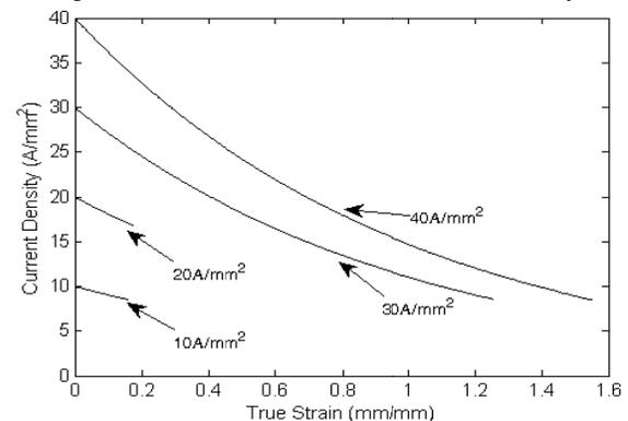
FIGURE 3. CURRENT DENSITY VARIES WITH STRAIN DURING TEST.
