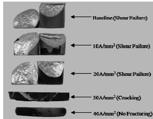
FIGURE 2. VISUAL SPECIMEN GEOMETRIES.
