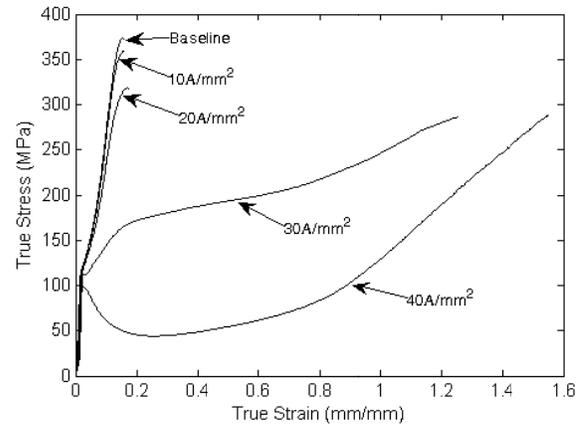
FIGURE 1. MAGNESIUM FLOW STRESS RESULTS.
