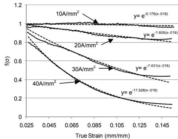
FIGURE 5. STRESS RATIO AS A FUNCTION OF STRAIN FOR VARIOUS CURRENT DENSITIES.
