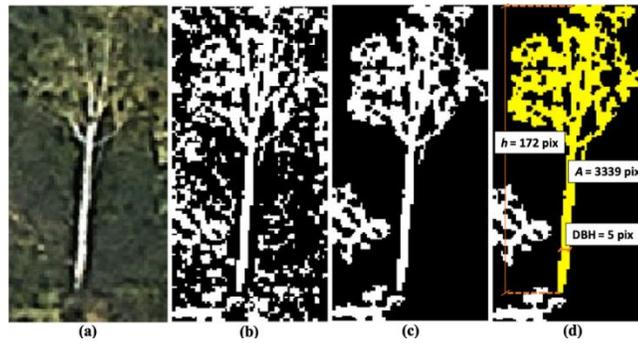
**Figure 1.** Extraction of tree pixels using image processing tools
